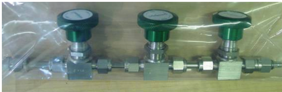
Figure 60. SS valves after vacuum bake.
