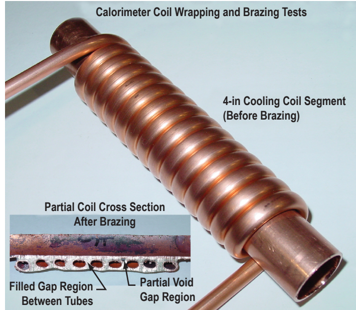
Figure 8. Brazing development testing for coil-type calorimeter design.
