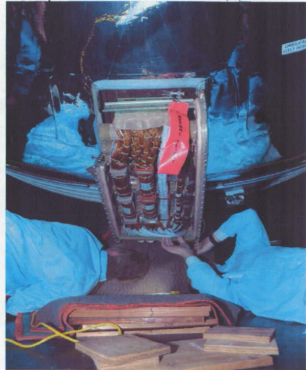
Pic 3: Engineers analyze umbilical wiring between Apollo Command Module's service and crew modules.
