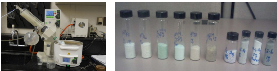
Figure 2.—(a) Assembly of a Büchi Rotavapor 210, a heating bath, and a Vacuum Pump (V-700) used to remove water from the photocatalyst. (b) Photocatalysts after the drying process in the rotovap, storage in a furnace and calcination at 400 °C.
