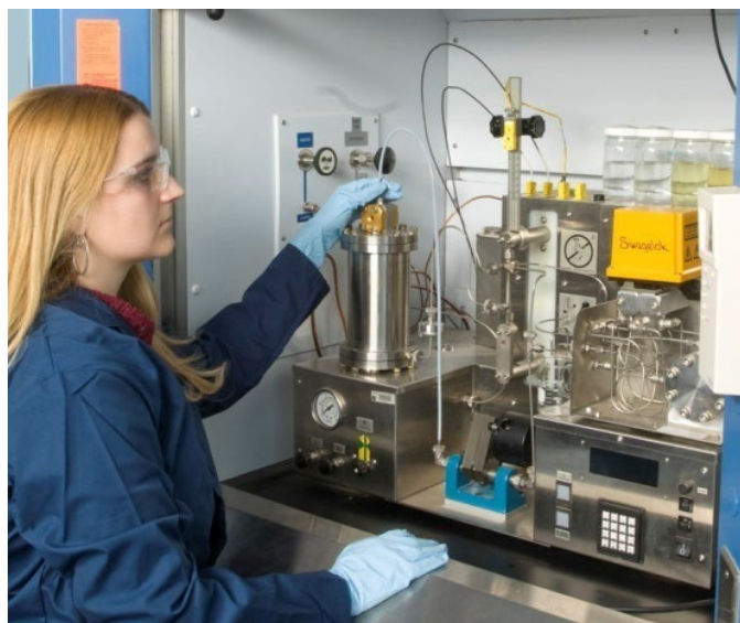
Figure 1.—Hot Liquid Process Simulator inside of fume hood in room 102.
