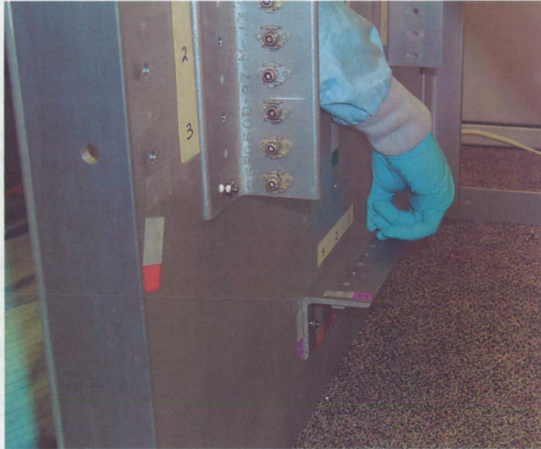
Figure 14. Technician installing screw into hole in group 3
