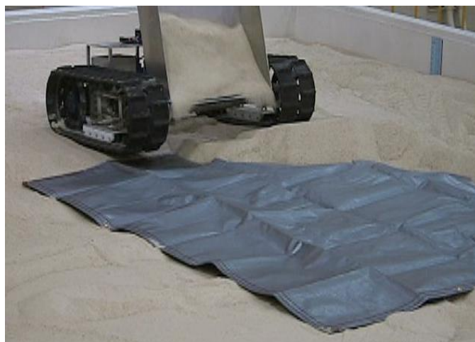
Figure 9.—Cratos burying a tarp with lunar simulant.
