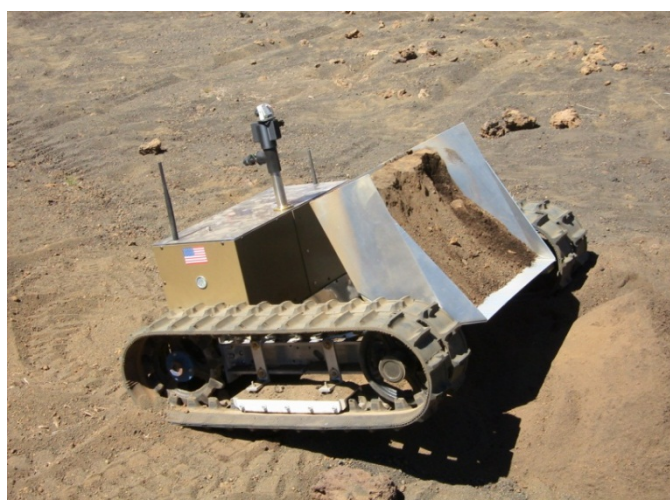
Figure 8.—Cratos moving volcanic soil on Hilo in Hawaii.
