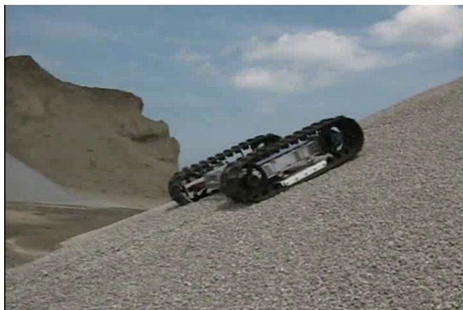
Figure 7.—Cratos ascending a steep grade on lunar simulant.
