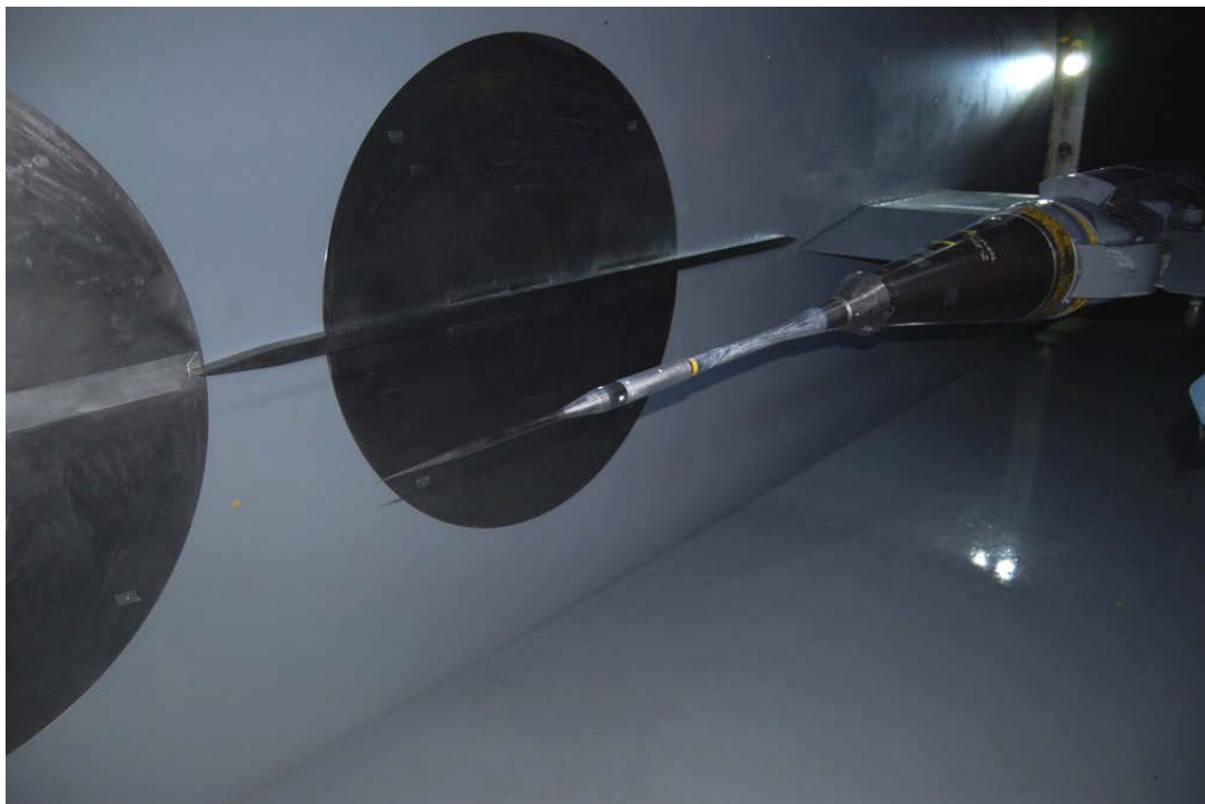
Figure 7.3-3. Photograph of the 2-in Sonic Boom Pressure Rail Installed in the NASA Ames 9' x 7' Test Section
