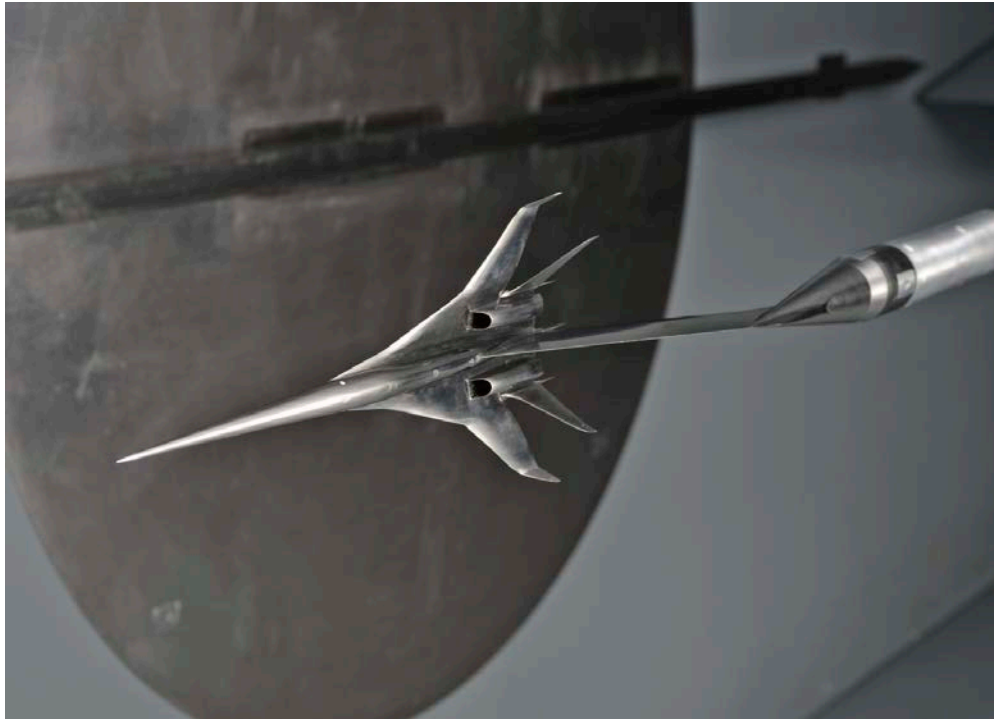
Figure 7.4-1. BM1 Model with VS2 Strut Installed in the NASA Ames 9' x 7' Wind Tunnel
