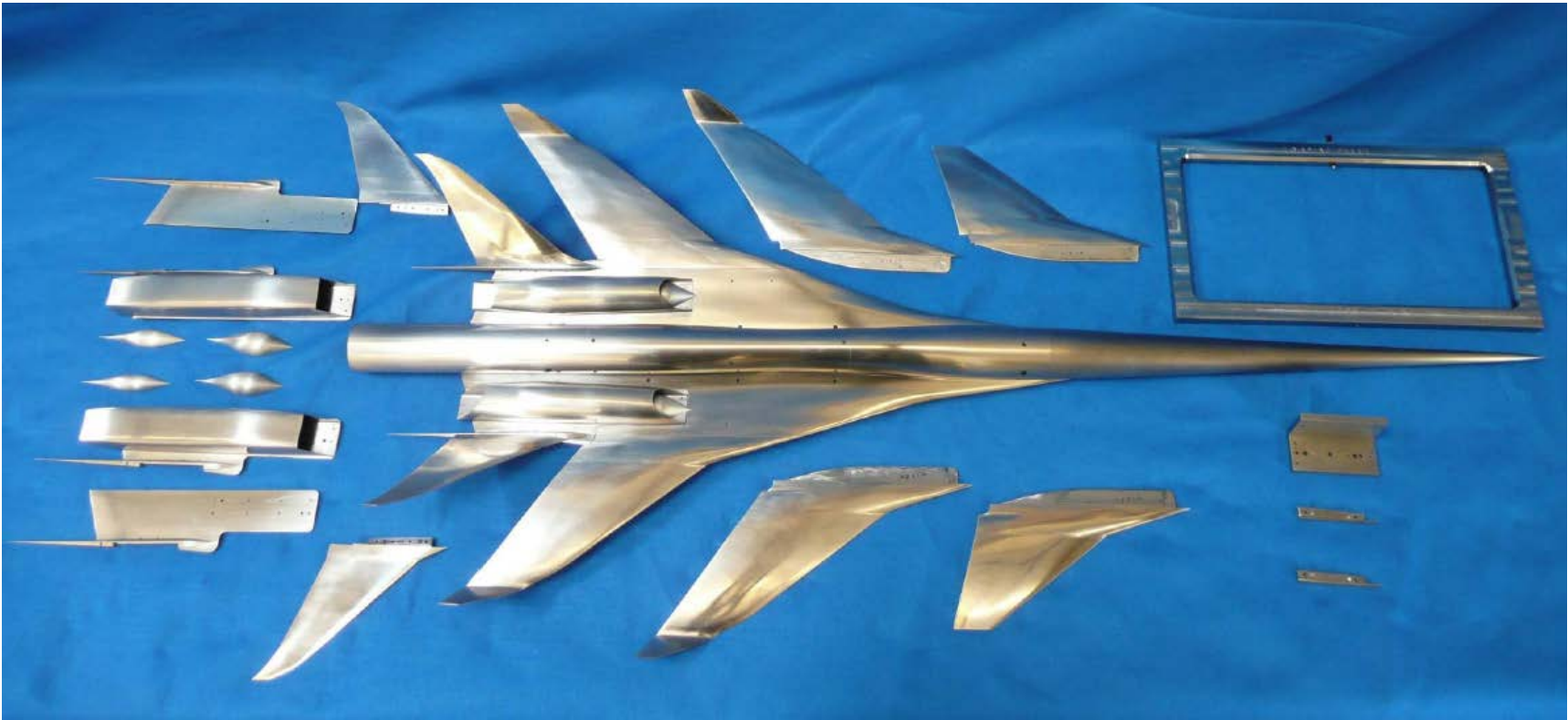
Figure 4.3-4. Performance Wind Tunnel Model and Associated Modular Part
