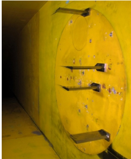
Figure 5.2-1. NASA Single Probes Used in the 2008 Sonic Boom Test
