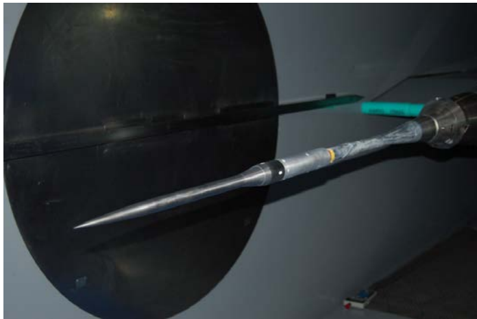
Figure 4.4-3. AS2 Model Installed in NASA Ames 9' x 7' Wind tunnel
