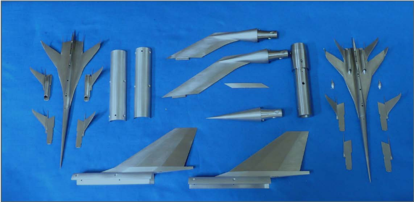
Figure 4.2-1. Boom Model 1 and Boom Model 2 and Associated Modular Hardware
