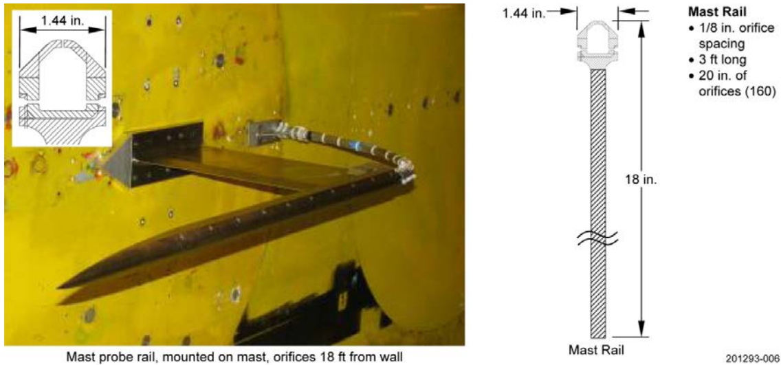
Figure 5.4-1. NASA Mast Rail Used in the 2008 Sonic Boom Test
