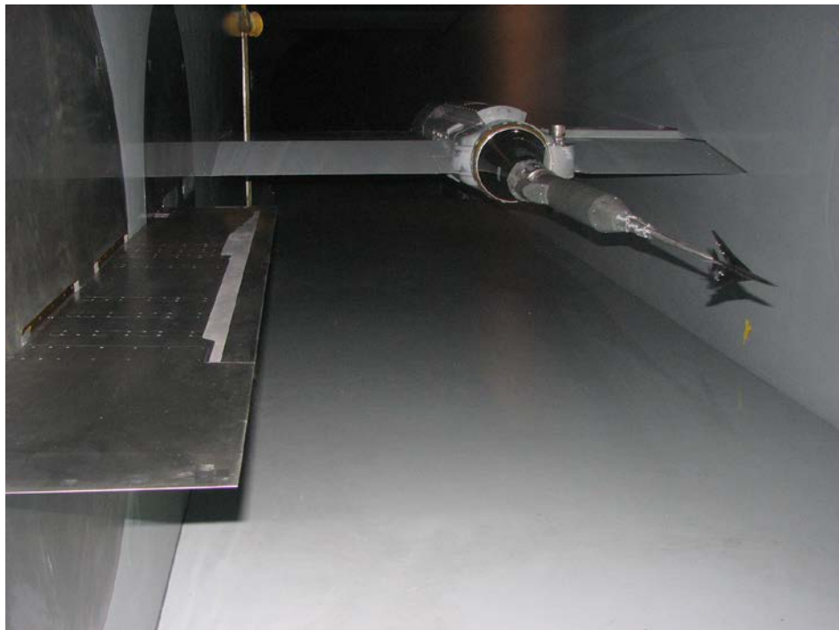
Figure 6.2-3. The 14" Blade Rail Installed in the NASA Ames 9' x 7' Wind Tunnel
