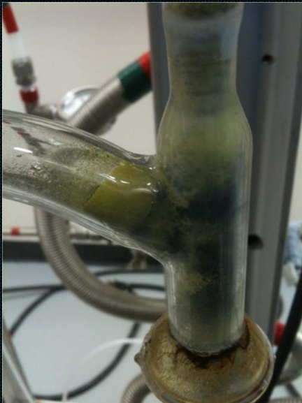
H 2 and WCl 6 /Ar mixture junction at reactor inlet
