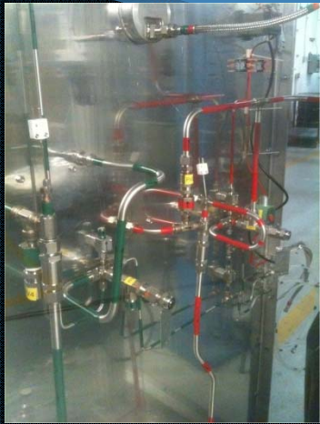
Gas line simplification, valve sequence, ball/socket joints
