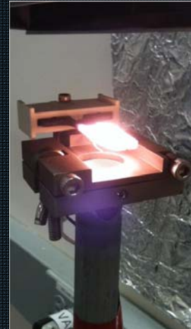
Burn-stack hinge & nichrome flame arrestor
