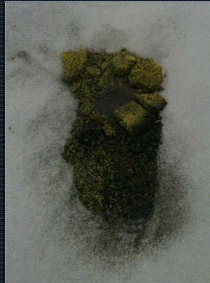
WCl 6 and W coated ZrO 2 blockage
