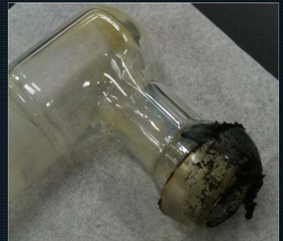
Sublimator outlet ball joint vacuum grease blow by location
