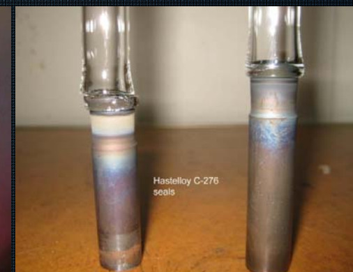
Failed C-276 Seal
