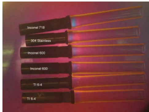
FIGURE 5. Polarized image of the heat induced strain on the glass-to-metal seals. Image courtesy of Larson Electronic Glass.
