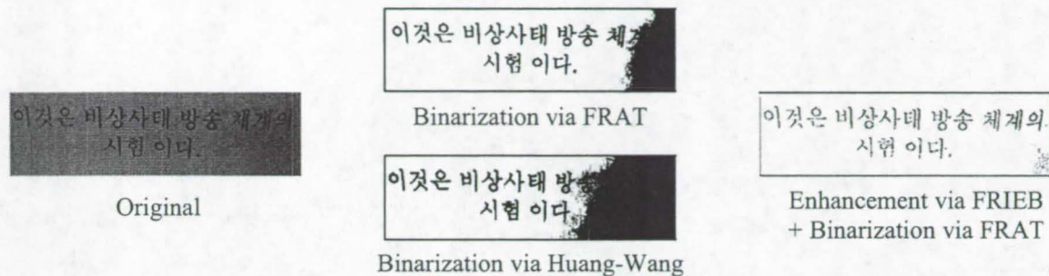
Figure 3. Effect of enhancing an image via FRIEB prior to binarization via FRAT and Huang-Wang techniques.
