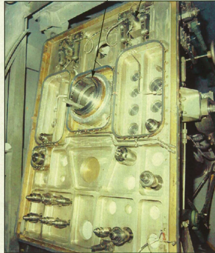
Shuttle LH2 Ground Side Umbilical
