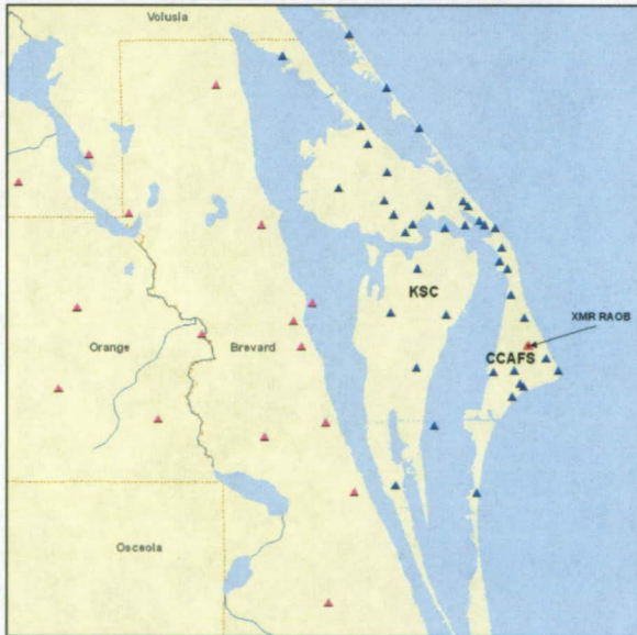
Figure 1. KSC/CCAFS wind tower network. Magenta triangles represent the mainland towers that may be eliminated. The XMR RAOB site is located at the red triangle.
