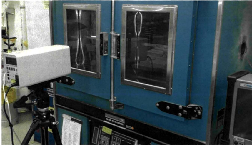
Figure 8: Test Setup with Laser Extensometer
