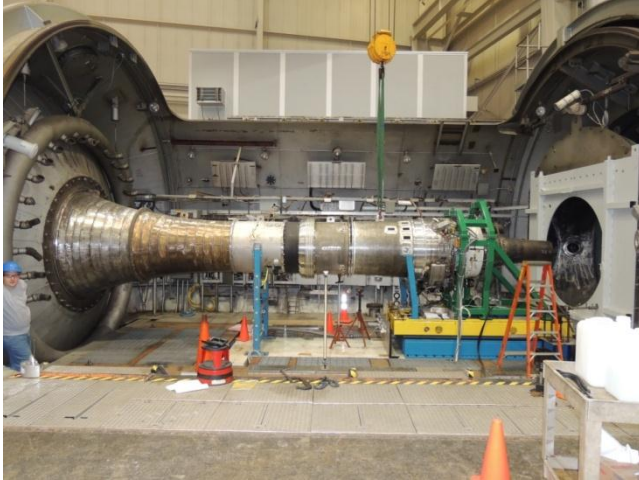
PSL Configured with the Honeywell ALF502 Engine Known to Ice
