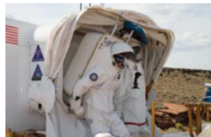
Figure 5 Suitport Testing The crew tested the new rear entry suits with the suitports on the lunar rover to minimize lunar dust exposure/contamination.
