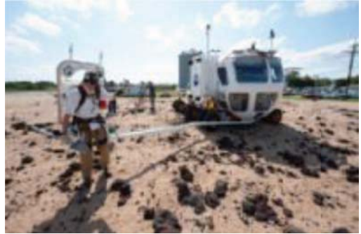
Figure 8 Simulated EVA with "Boom" Concept Testing of an EVA at a low/zero-G gravity asteroid using a rover to simulate the spacecraft and a boom to place the crewmember near the asteroid surface.
