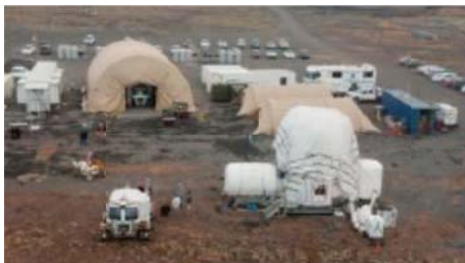
Figure 7 DRATS 2011 Deployment at Black Point Lava Flow Lunar Electric Rover and Deep Space Habitat prototypes shown in foreground with inflatable support facilities in the background.
