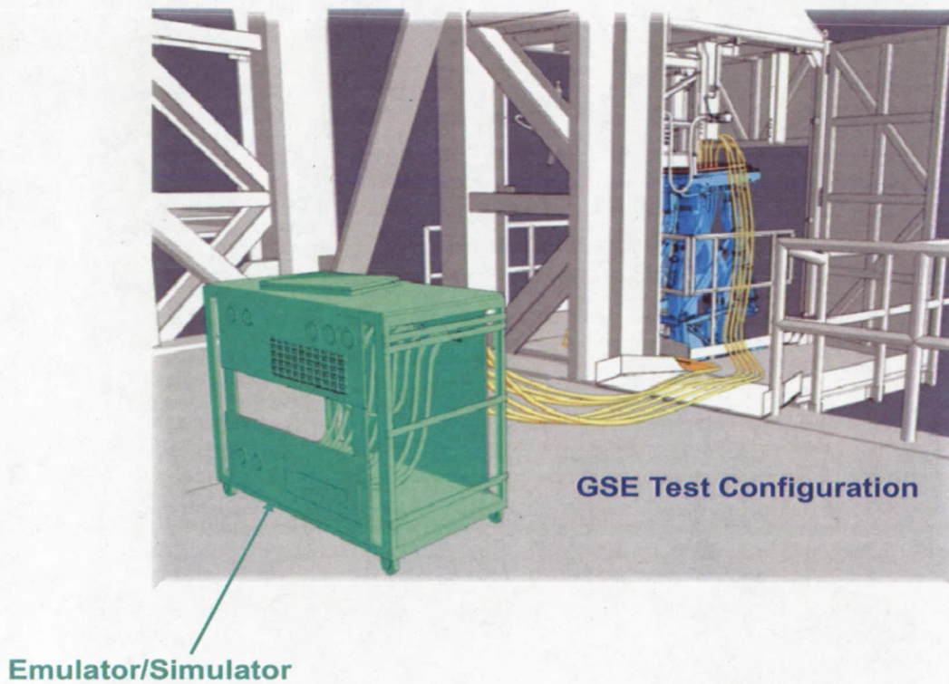
Figure 7, Emulators/Simulators Attached to Flight Umbilical Plates
