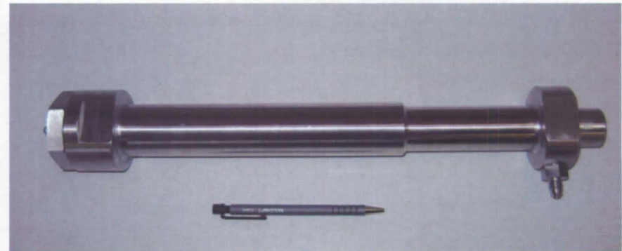
Reactor Vessel (note pen for scale)
