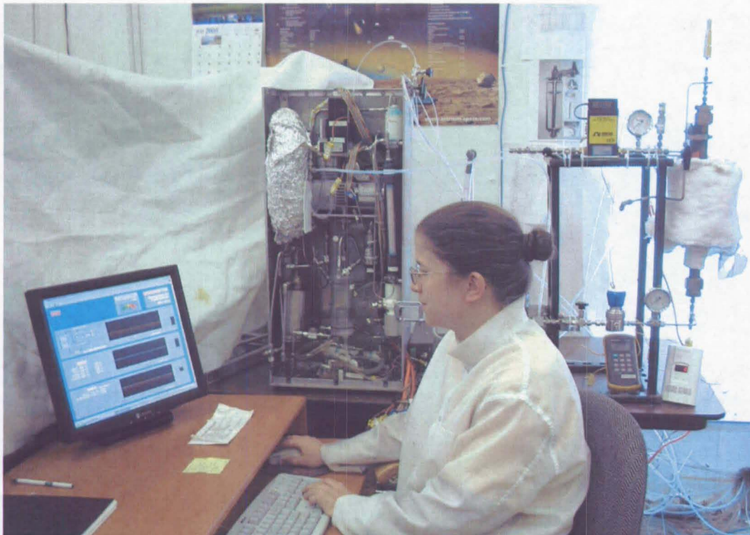
Integrated COSRS-RWGS-Electrolyzer System During Operation.
