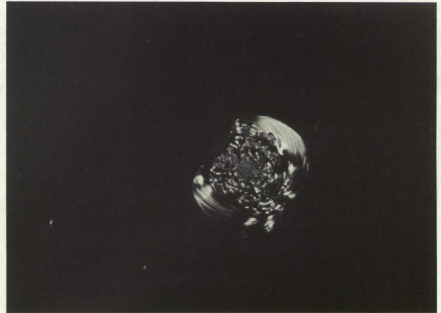
An Orbiter Window Defect
