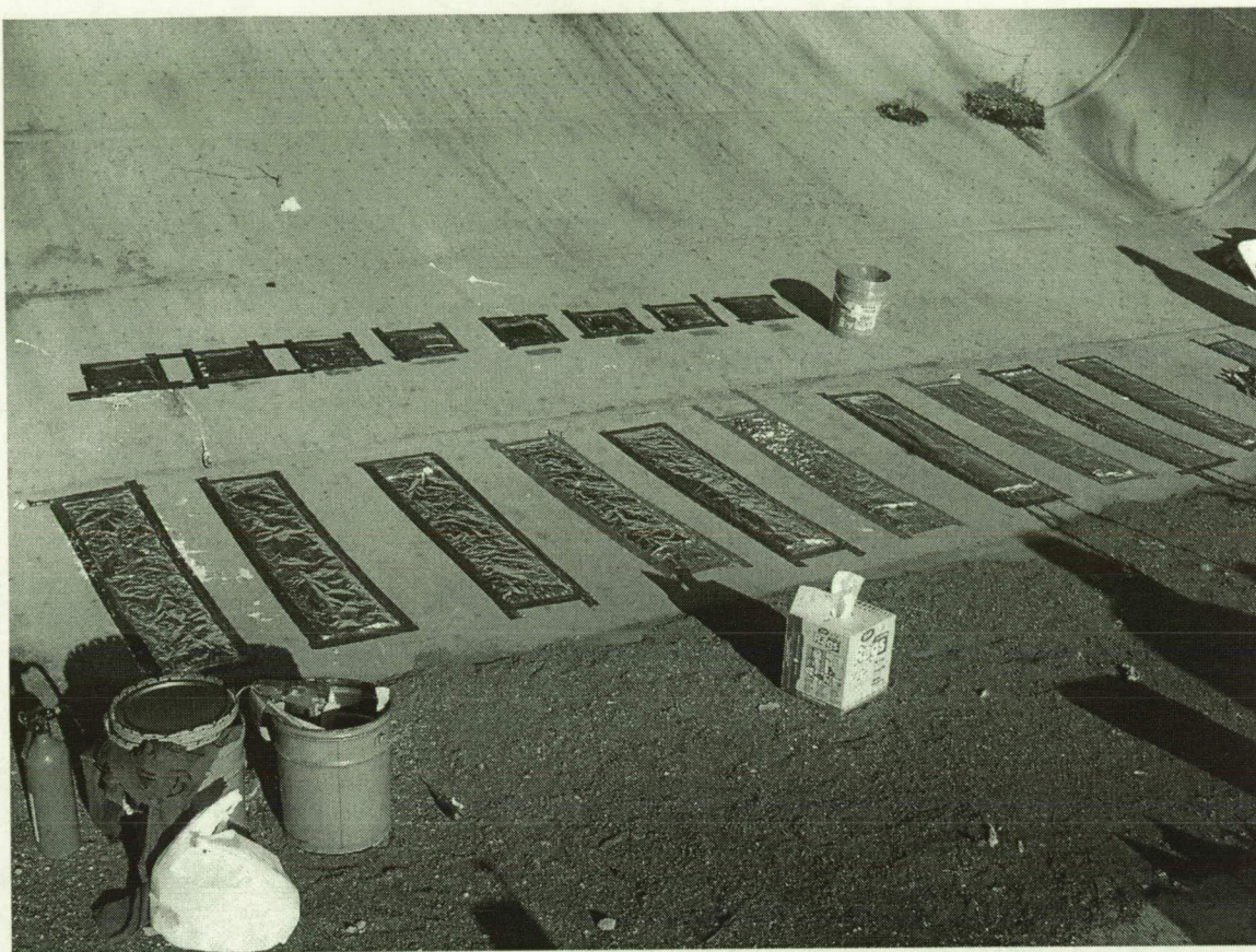
FIGURE 4. Photograph of BTS test panels covered with aluminum foil or copper sheets.
