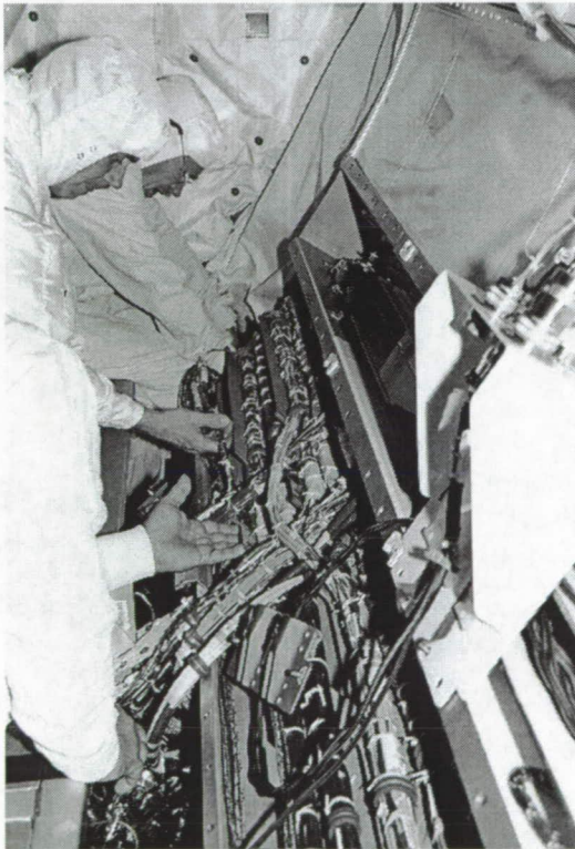
Figure 1. The Space Shuttle Orbiter has over 200 miles of wiring.
