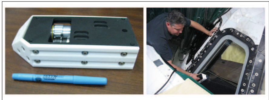
The Surface Inspection Tool (left), shown in use (right). The handle was added to accommodate smaller hands and reduce user fatigue.
