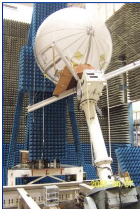
Prototype Inflatable Radome Antenna System at GRC
