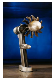
Open rotor testing in GRC 9 x 15 Low Speed Wind Tunnel (General Electric Aviation)
