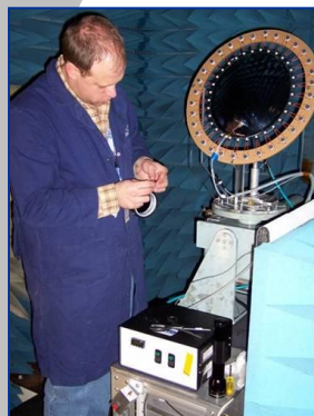
0.3 meter prototype Membrane reflector
