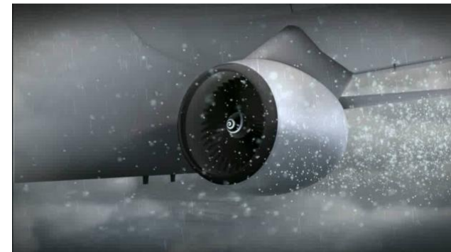
Artist rendition of the engine icing accumulation and shedding.
