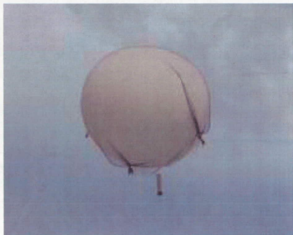
Figure 13: Tethered Weather Balloon utilized in Recovery Systems Drop Tests and Validation of Ram Air Parachute
