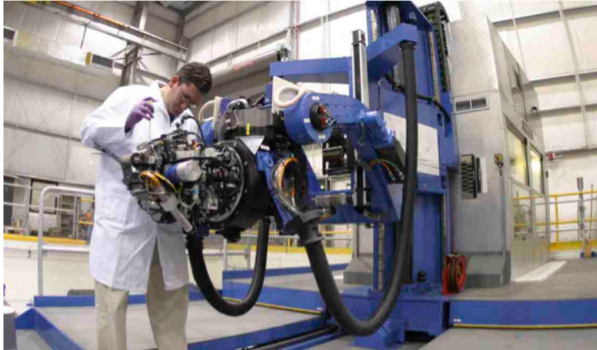
Figure 1. Fiber placement system (Lockheed Martin)
