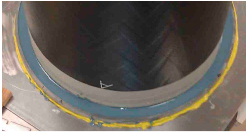
Figure 7. Potted end of tow-steered shell
