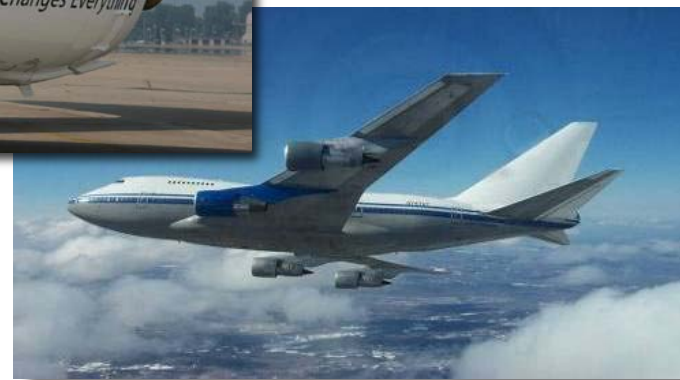
GTF Demonstrator Engine Installed on P&W 747 Test-bed Aircraft ('08)
