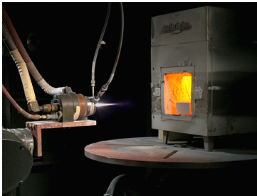
Plasma-spray processing of Environmental barrier coatings for various components
