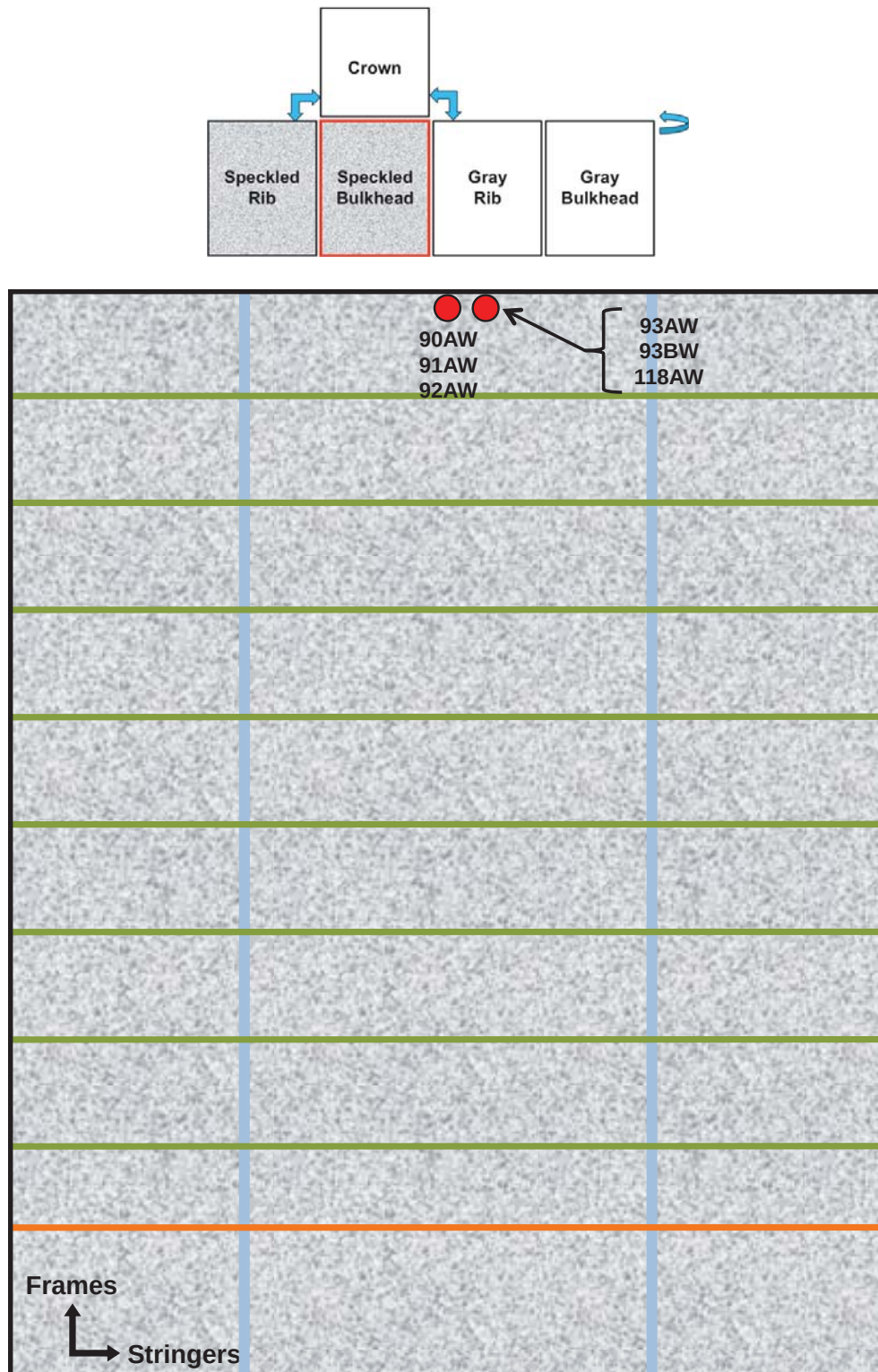
Figure 12. Speckled bulkhead strain gage locations.
