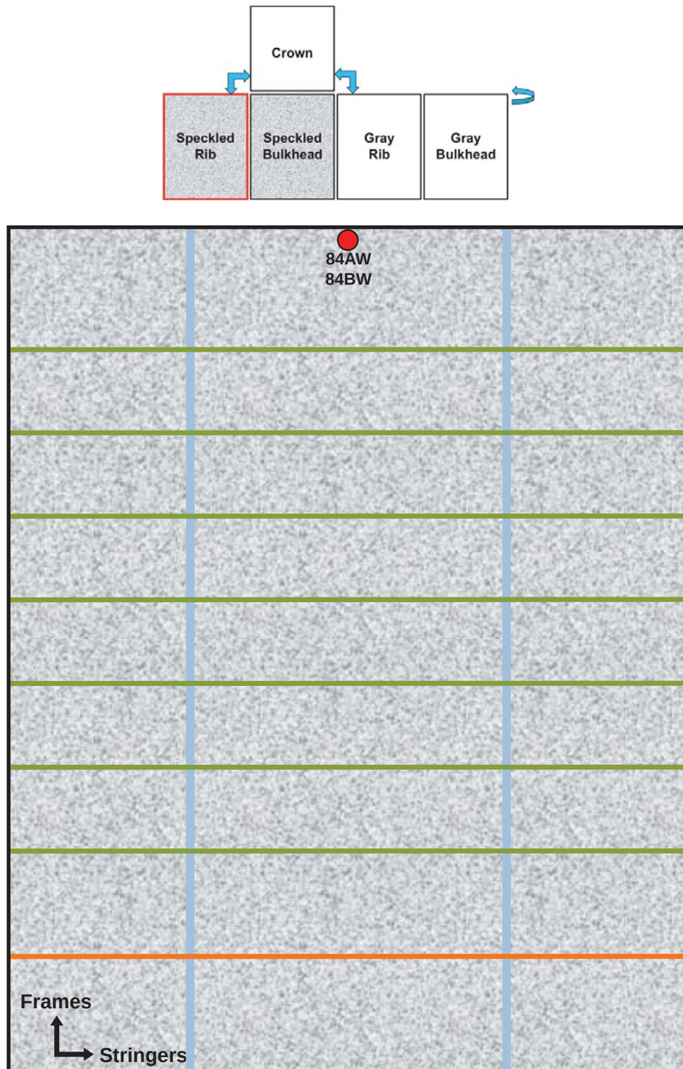
Figure 11. Speckled rib strain gage locations.
