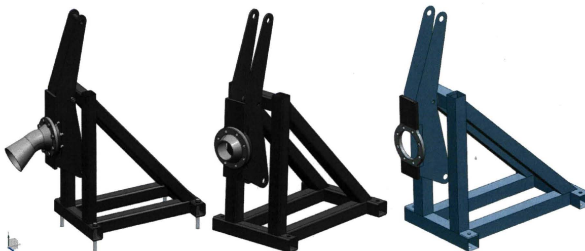
Figure 2. Process of simplifying the geometry of the structure to decrease run time.
