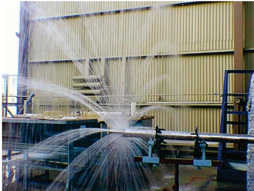
Figure 4. Spray bar water flow test at Boeing.
