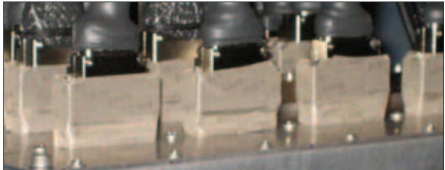
Figure 2. This picture shows the Implemented Design Concept . Conductive tape is wrapped starting with the pedestal, around the D connector, and ending at the cable backshell. This provides a continuous conductive enclosure that seals potential RF leakages from between the D connector and the chassis, and from between the cable plug and the connector receptacle.
