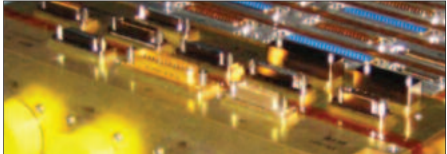
Figure 1. This picture shows the Design Concept , with the pedestals and the chassis as one piece of metal. The D-sub or Micro-D connector is then mounted on the pedestal. This pedestal provides a few extra millimeters for the conductive tape to make contact with the chassis.
