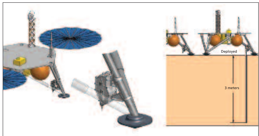
The Next-Generation Heat Flow Probe Concept. At left, the conceptual design of the heat flow probe mounted on the spacecraft landing system; at right, deployment of the heat flow probe.
