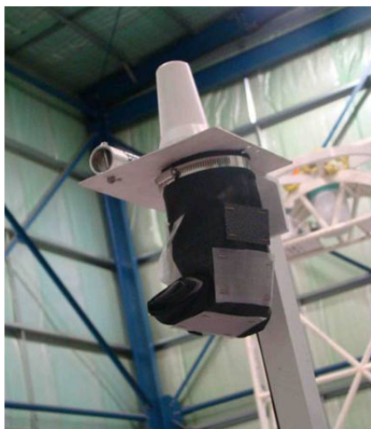
Figure 3.—The flight cassette is fixed on the metal bar of the GPS antenna of the payload. The control sample, which appears dark in the picture, has been cured prior to the flight and is not covered with a Teflon mesh.
