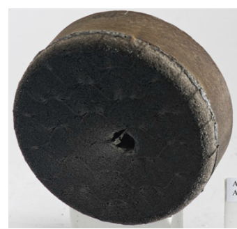
Figure 11 – Space Environmental Effects Testing – simulated micrometeoroid impact followed by arc jet testing
