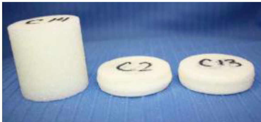
Figure 8 – Closed-Cell Foams Before (C14) and After (C2 and C13) Impact Testing
