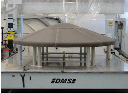
Figure 10 – Milling of 2.65-m aeroshell to demonstrate manufacturability
