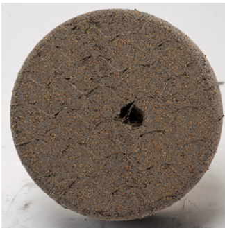
Figure 11 – Space Environmental Effects Testing – simulated micrometeoroid impact followed by arc jet testing
