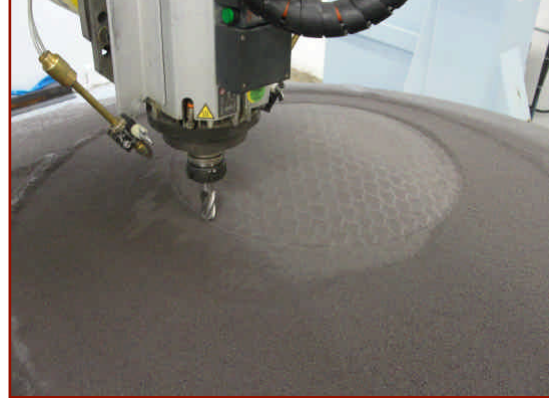
Figure 10 – Milling of 2.65-m aeroshell to demonstrate manufacturability
