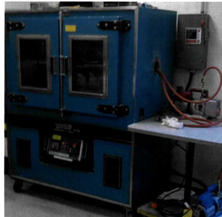
Oven Cure of Panel Under Vacuum
