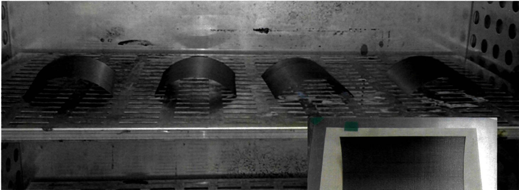
Panels in the oven for a free standing post cure
