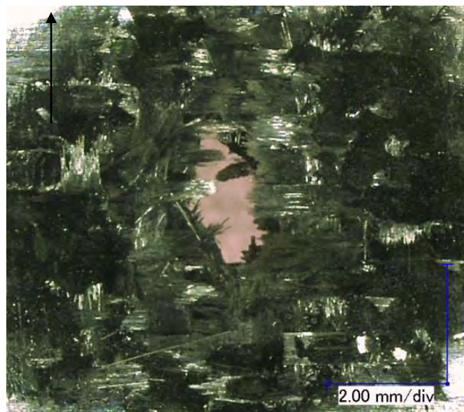
Figure 433 Close-up View of Most Significant Damage to Back Side of NP 504 Substrate (black arrow indicates flight path of projectile / damage within red circle in Figure 247)
