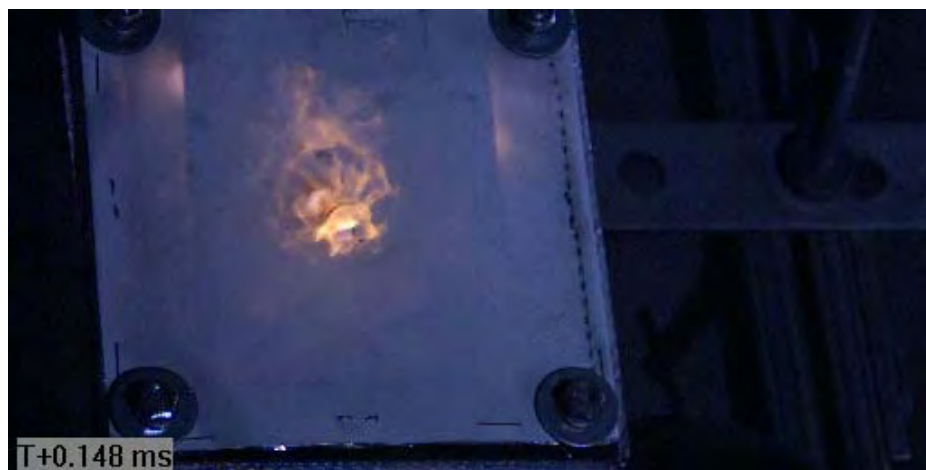
Figure C44 Projectile Impacting Target (via Phantom v711)
