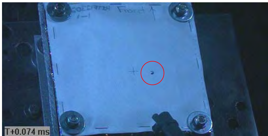
Figure C61 Image of Projectile Captured Prior to Impact (via Phantom v711 / projectile within red circle)
