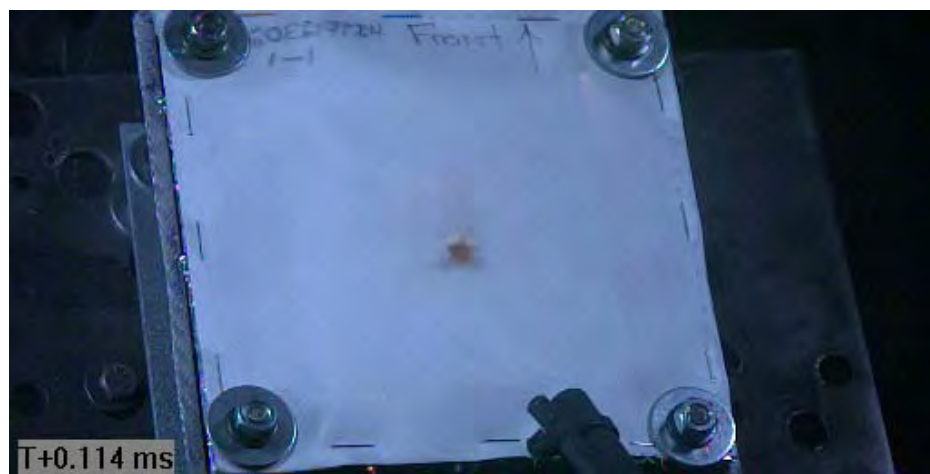
Figure C62 Projectile Impacting Target (via Phantom v711)
