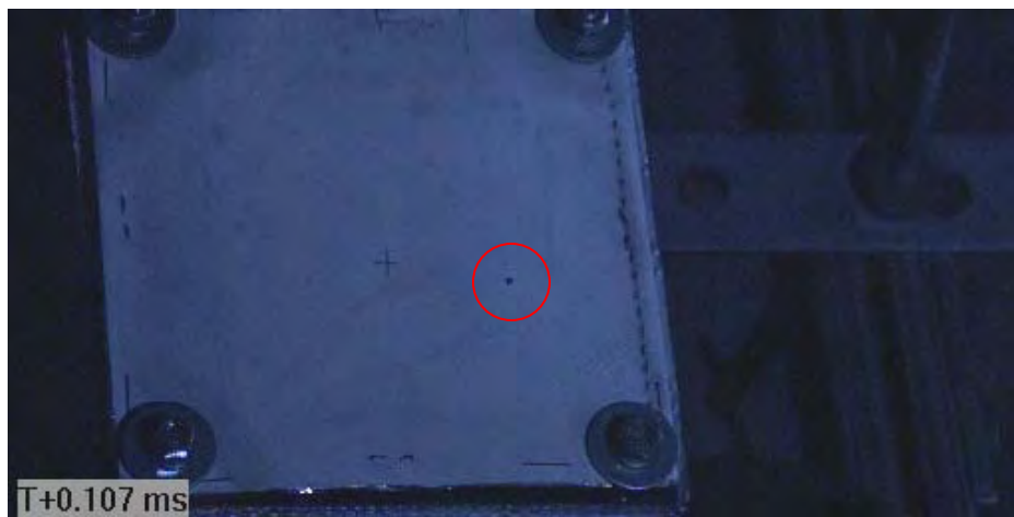
Figure C43 Image of Projectile Captured Prior to Impact (via Phantom v711 / projectile within red circle)
