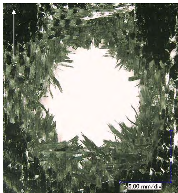
Figure 554 Close-up View of Most Significant Damage to Back Side of NP 504 Substrate (black arrow indicates flight path of projectile / damage within red circle in Figure 584)
