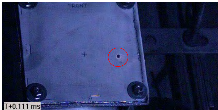
Figure C72 Image of Projectile Captured Prior to Impact (via Phantom v711 / projectile within red circle)
