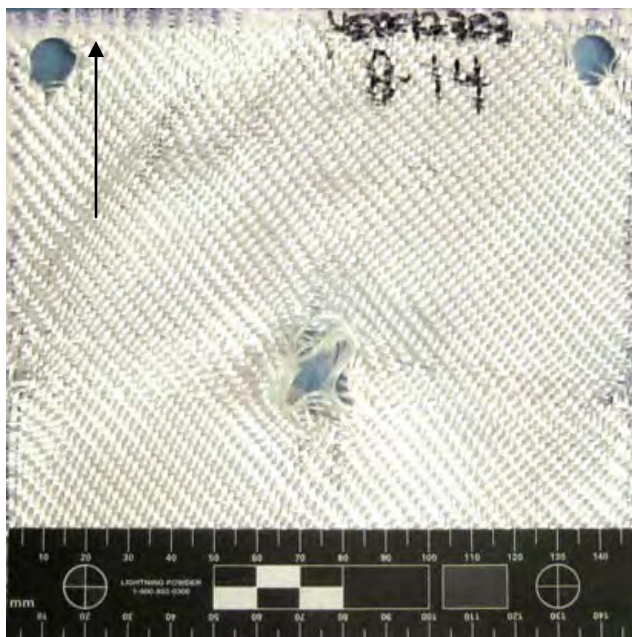
Figure 348 Overall View of Damage to Back Side of Last Fiberglass Layer (scale in 5mm increments / black arrow indicates flight path of projectile)
