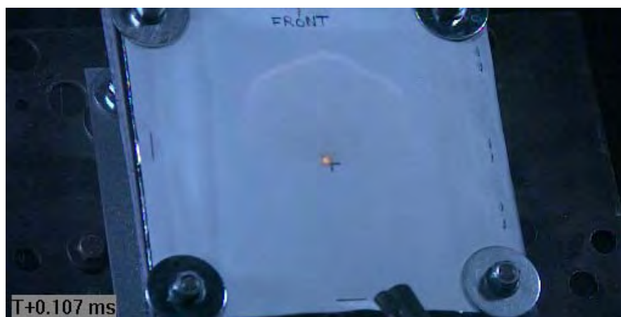
Figure C85 Image of Projectile Impacting Target (via Phantom v711)
