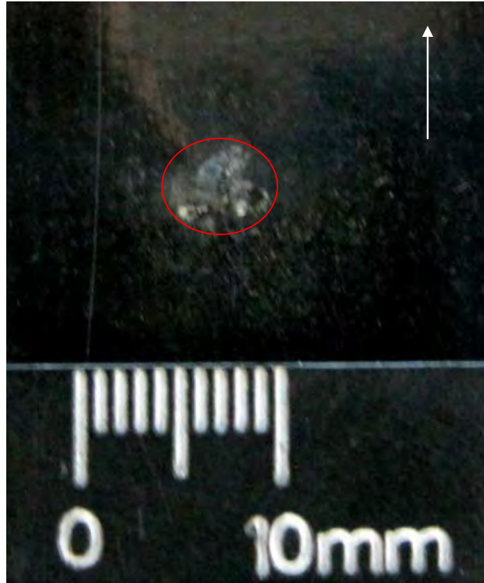
Figure 46 Close-up View of Damage to Back Side of NP 504 Substrate (scale in 1mm increments / white arrow indicates flight path of projectile)
