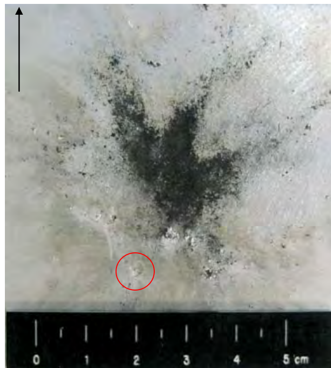
Figure 482 Close-up View of Damage to Front of Rear Wall (scale in 5mm increments / black arrow indicates flight path of projectile)
