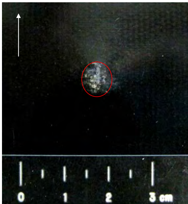
Figure 496 Close-up View of Damage to Back Side of NP 504 Substrate (scale in 5mm increments / white arrow indicates flight path of projectile)
