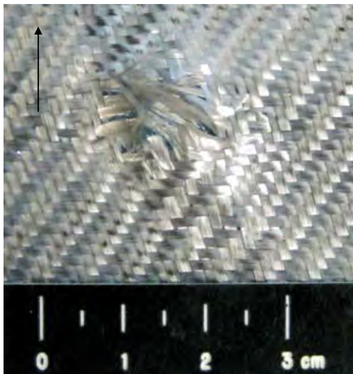
Figure 80 Close-up View of Damage to Back Side of Last Fiberglass Layer (scale in 5mm increments / black arrow indicates flight path of projectile)
