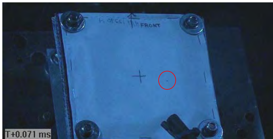
Figure C22 Image of Projectile Captured Prior to Impact (via Phantom v711 / projectile within red circle)
