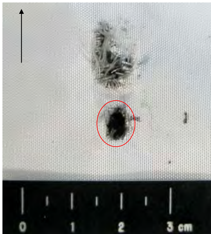
Figure 441 Close-up View of Damage to Front of MLI (scale in 5mm increments / black arrow indicates flight path of projectile / projectile impacted within red circle)
