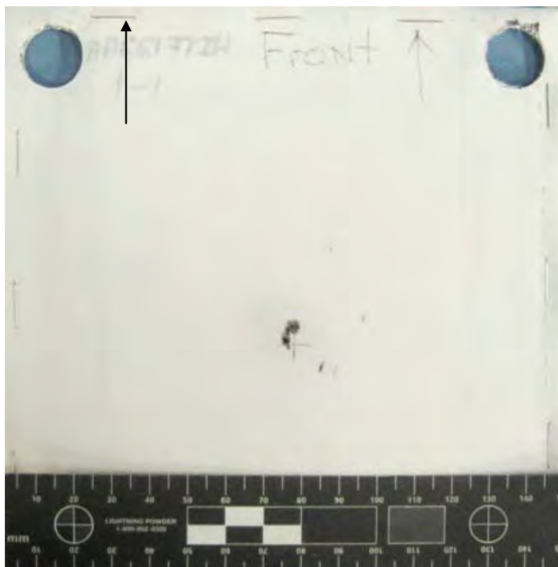
Figure 279 Overall View of Damage to Front of MLI (scale in 5mm increments / black arrow indicates flight path of projectile)
