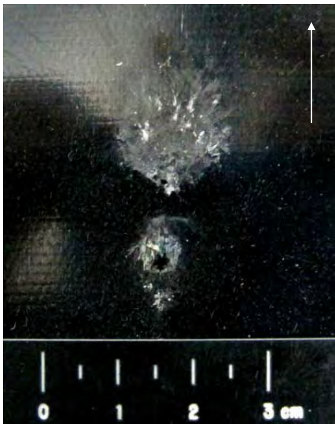
Figure 93 Close-up View of Damage to Front of NP 504 Substrate (scale in 5mm increments / white arrow indicates flight path of projectile)
