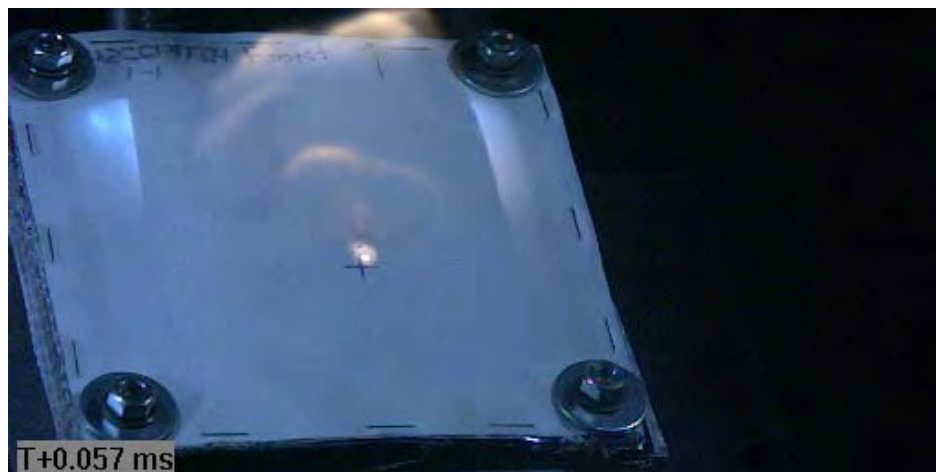
Figure C6 Projectile Impacting Target (via Phantom v711)
