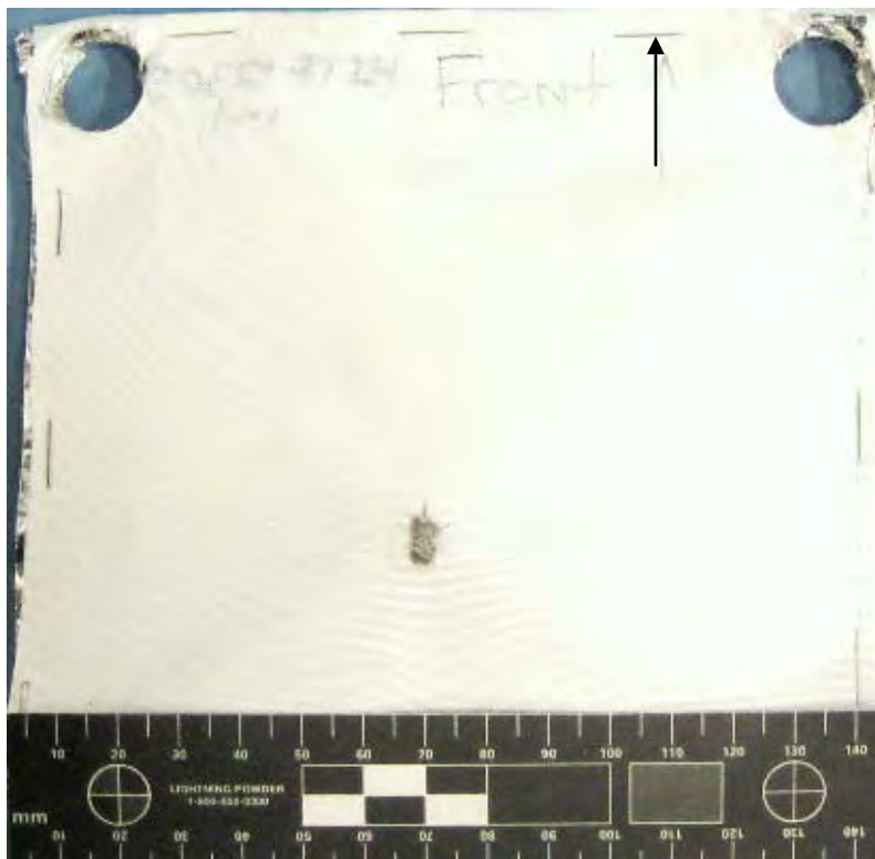
Figure 339 Overall View of Damage to Front of MLI (scale in 5mm increments / black arrow indicates flight path of projectile)
