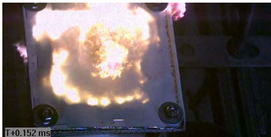
Figure C73 Projectile Impacting Target (via Phantom v711)
