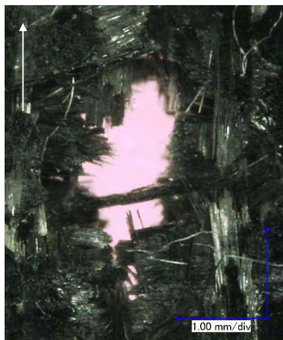
Figure 193 Close-up View of Most Significant Damage to Back Side of NP 504 Substrate (white arrow indicates flight path of projectile / damage within red circle in Figure 192)
