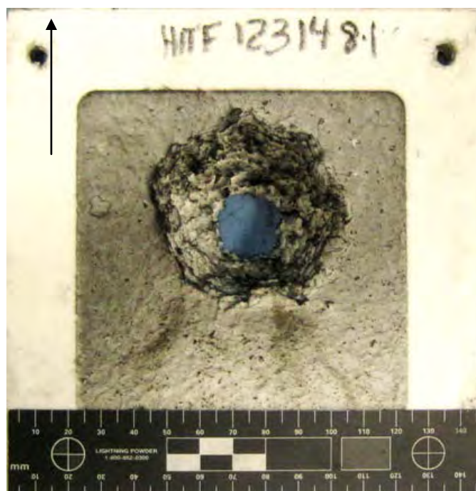
Figure 579 Overall View of Damage to Back Side of Saffil Layer (scale in 5mm increments / black arrow indicates flight path of projectile)
