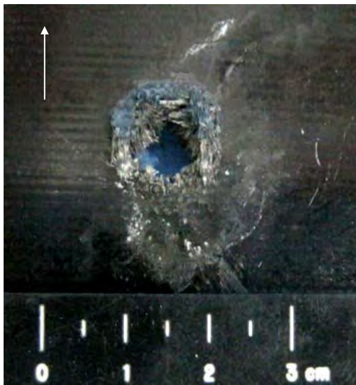
Figure 239 Close-up View of Damage to Front of NP 504 Substrate (scale in 5mm increments / white arrow indicates flight path of projectile)
