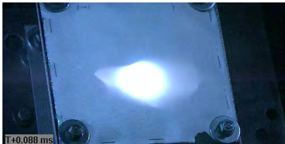
Figure C20 Projectile Impacting Target (via Phantom v711)
