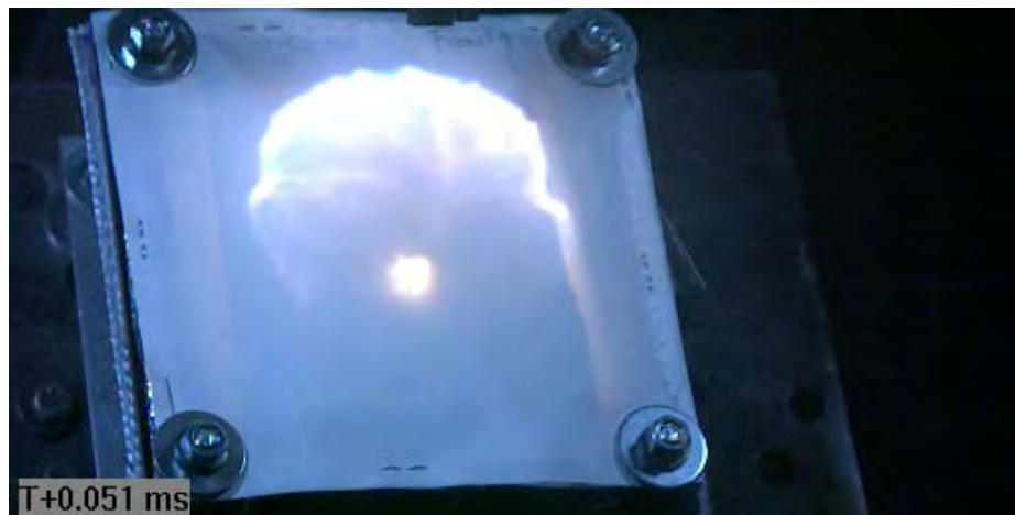
Figure C56 Projectile Impacting Target (via Phantom v711)
