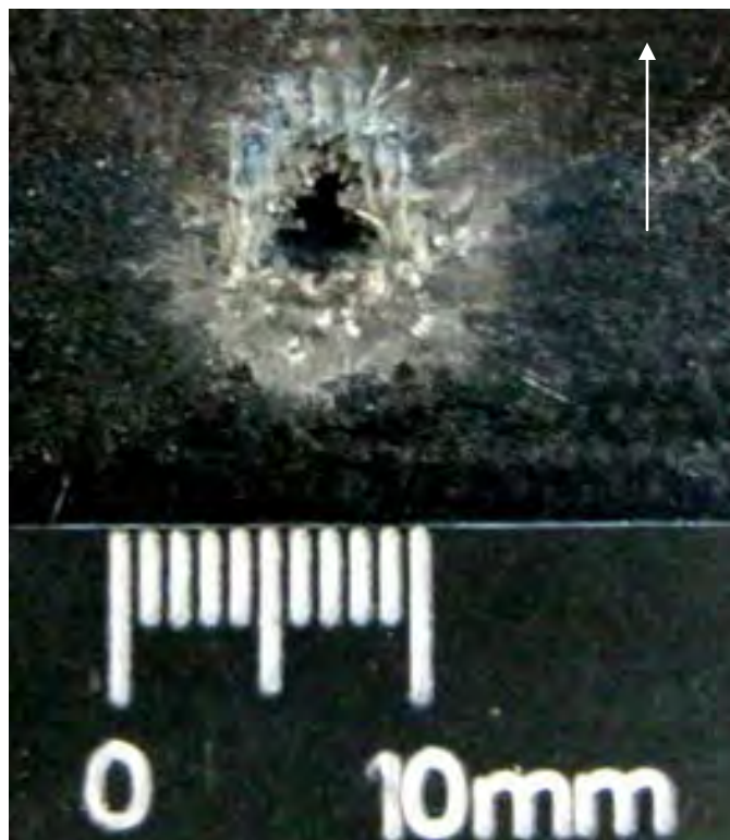
Figure 460 Close-up View of Damage to Front of NP 504 Substrate (scale in 1mm increments / white arrow indicates flight path of projectile)
