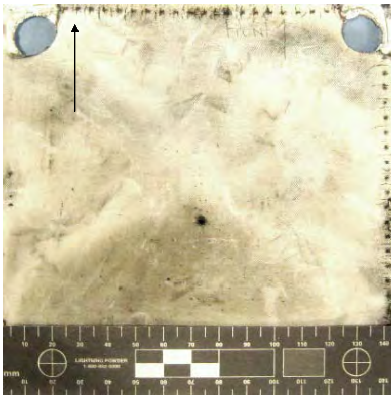
Figure 504 Overall View of Damage to Front of MLI (black arrow indicates flight path of projectile / scale in 5mm increments)
