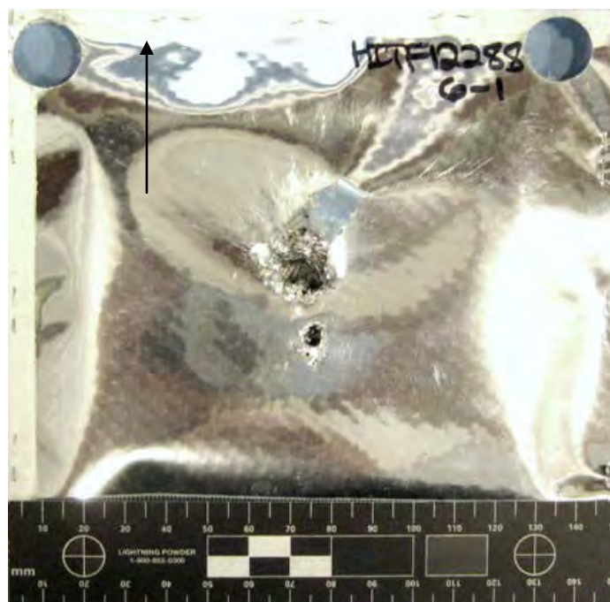
Figure 90 Overall View of Damage to Back Side of MLI (scale in 5mm increments / black arrow indicates flight path of projectile)
