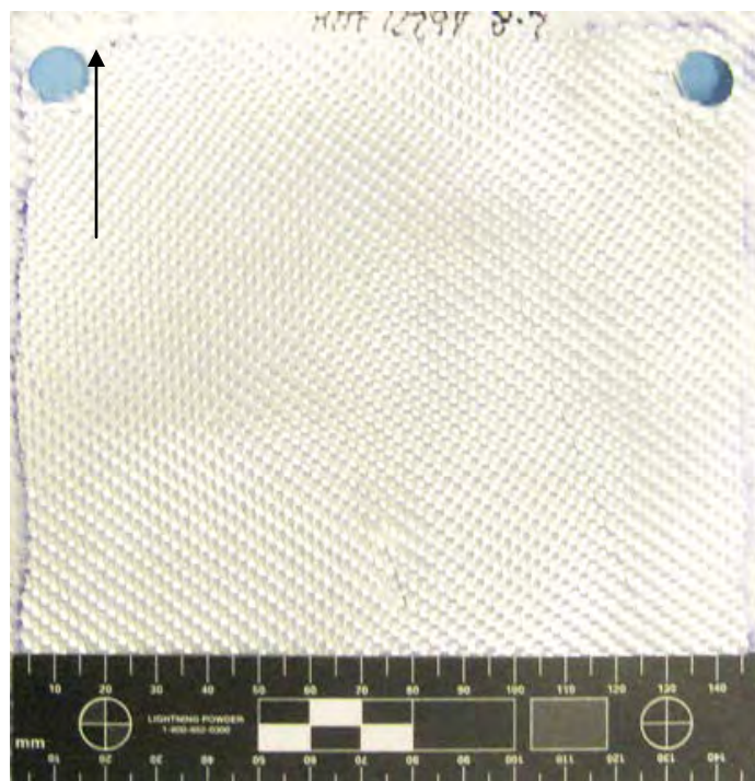
Figure 195 Overall View of Damage to Back Side of 7 th Fiberglass Layer (scale in 5mm increments / black arrow indicates flight path of projectile)
