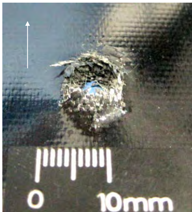
Figure 329 Close-up Oblique Side View of Damage to Back Side of NP 504 Substrate (scale in 1mm increments / white arrow indicates flight path of projectile)
