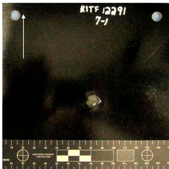
Figure 146 Overall View of Damage to Back Side of NP 504 Substrate (scale in 5mm increments / white arrow indicates flight path of projectile)
