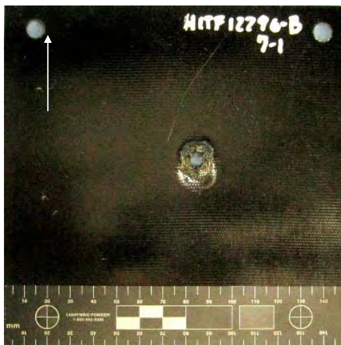
Figure 240 Overall View of Damage to Back Side of NP 504 Substrate (scale in 5mm increments / white arrow indicates flight path of projectile)
