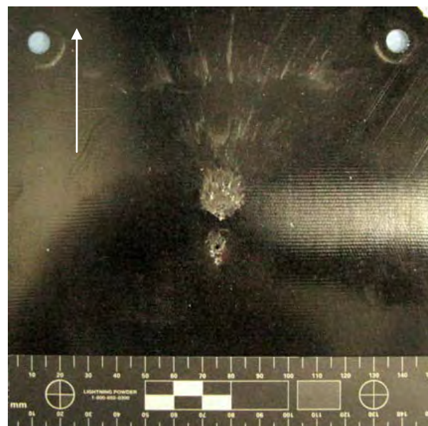
Figure 92 Overall View of Damage to Front of NP 504 Substrate (scale in 5mm increments / white arrow indicates flight path of projectile)
