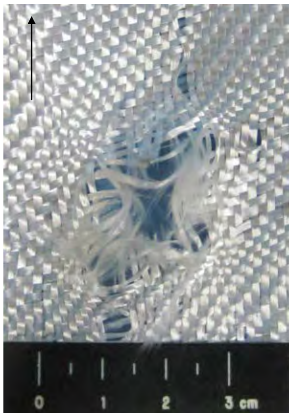
Figure 226 Close-up View of Damage to Back Side of Last Fiberglass Layer (scale in 5mm increments / black arrow indicates flight path of projectile)
