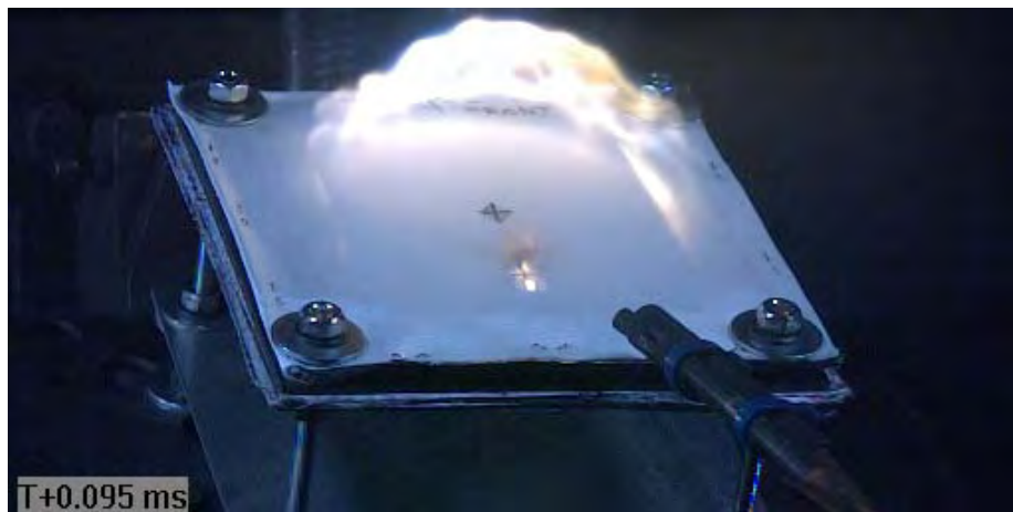
Figure C35 Projectile Impacting Target (via Phantom v711)
