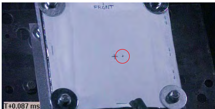
Figure C84 Image of Projectile Captured Prior to Impact (via Phantom v711 / projectile within red circle)
