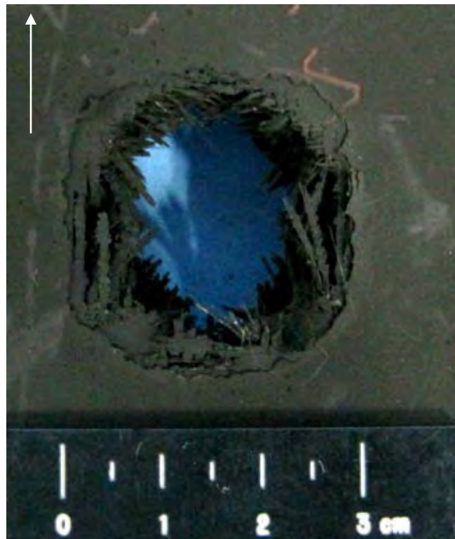
Figure 528 Close-up View of Damage to Front NP 504 Substrate with TORLON 5030 Delaminated (scale in 5mm increments / white arrow indicates flight path of projectile)
