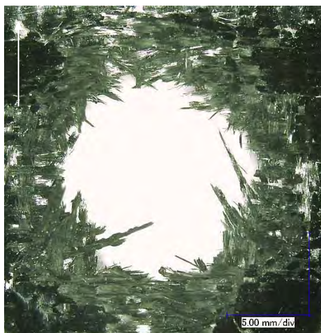
Figure 575 Close-up View of Most Significant Damage to Back Side of NP 504 Substrate (black arrow indicates flight path of projectile / damage within red circle in Figure 574)
