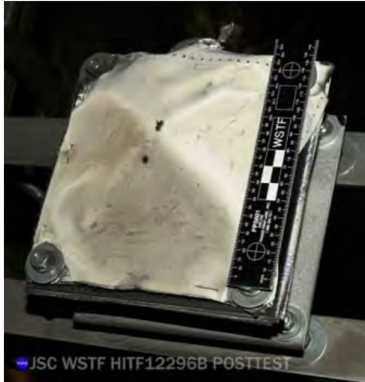
Figure 231 Overall View of Sample in the Target Tank (post-test)
