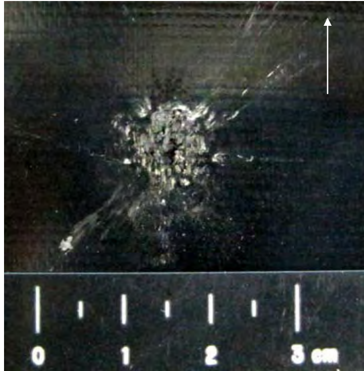
Figure 362 Close-up View of Damage to Front of NP 504 Substrate (scale in 5mm increments / white arrow indicates flight path of projectile)
