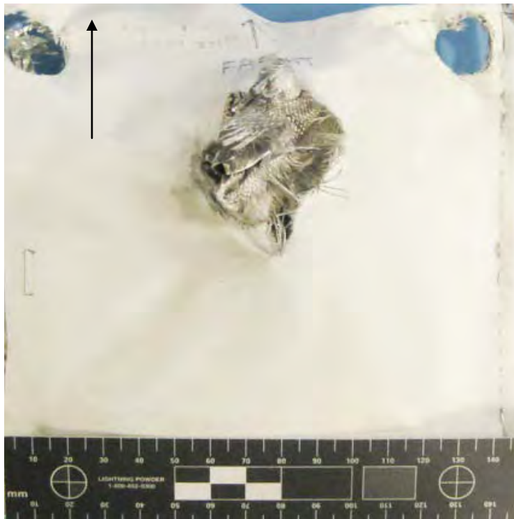
Figure 470 Overall View of Damage to Front of MLI (scale in 5mm increments / black arrow indicates flight path of projectile)
