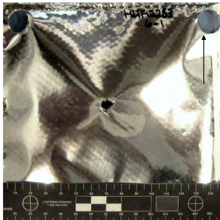
Figure 13 Overall View of Damage to Back Side of MLI (scale in 5mm increments / black arrow indicates flight path of projectile)
