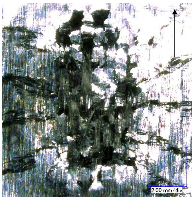
Figure 62 Close-up View of Most Significant Damage to Back Side of NP 504 Substrate (black arrow indicates flight path of projectile / damage within red circle in Figure 61)
