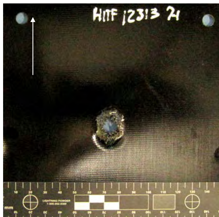
Figure 552 Overall View of Damage to Back Side of NP 504 Substrate (scale in 5mm increments / white arrow indicates flight path of projectile)
