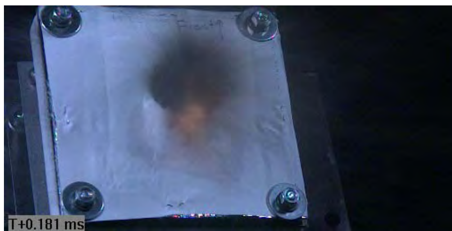
Figure C100 Image of Projectile Impacting Target (via Phantom v711)
