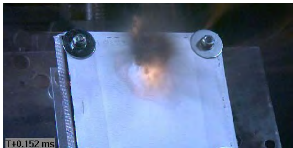
Figure C88 Image of Projectile Impacting Target (via Phantom v711)
