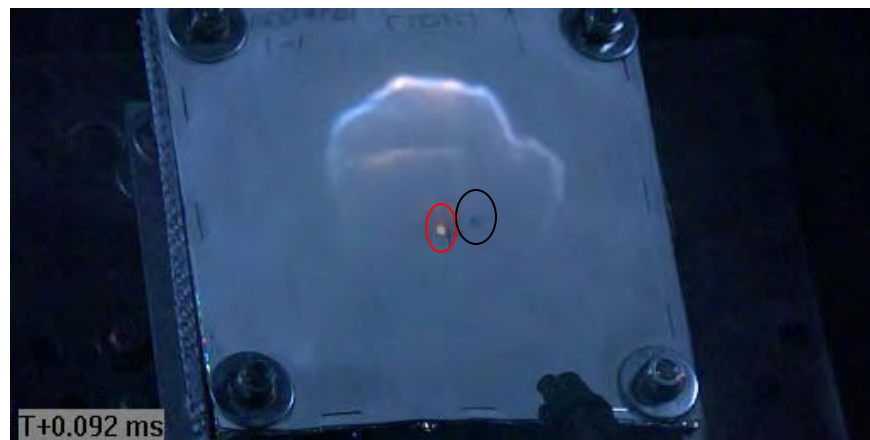
Figure C53 Image of Projectile Impacting Target and Secondary Debris Just Prior to Impacting Target (via Phantom v711 / projectile impacting within red circle / secondary debris within black circle and impacted directly above projectile entry damage)
