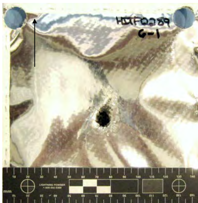
Figure 109 Overall View of Damage to Back Side of MLI (scale in 5mm increments / black arrow indicates flight path of projectile)
