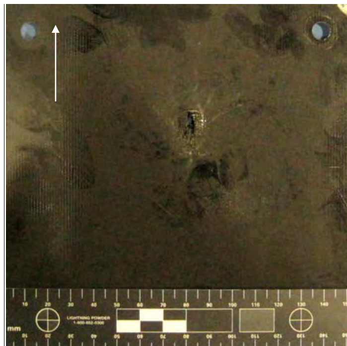
Figure 73 Overall View of Damage to Front of NP 504 Substrate (scale in 5mm increments / white arrow indicates flight path of projectile)
