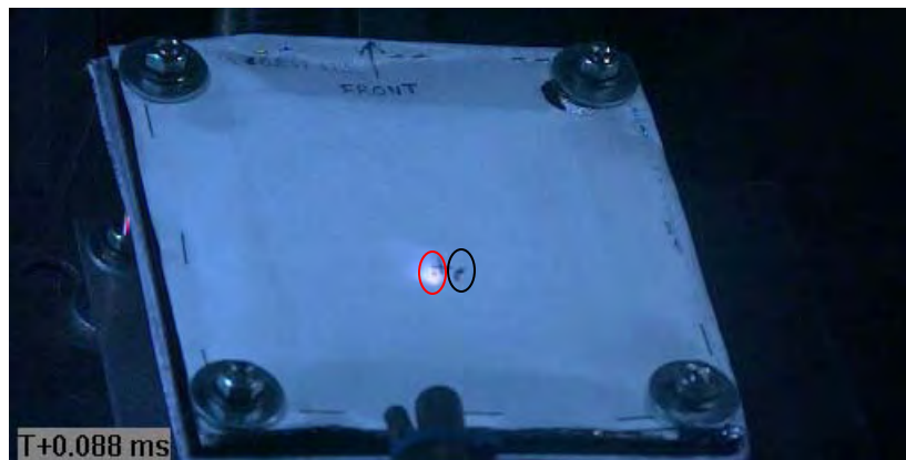
Figure C70 Image of Projectile Impacting Target and Secondary Debris Just Prior to Impacting Target (via Phantom v711 / projectile impacting within red circle / secondary debris within black circle and impact directly behind projectile entry damage)
