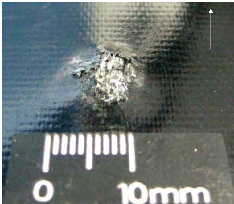
Figure 366 Close-up Oblique Side View of Damage to Back Side of NP 504 Substrate (scale in 1mm increments / white arrow indicates flight path of projectile)
