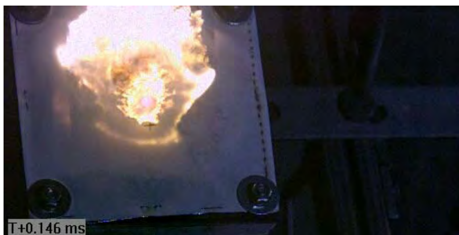
Figure C103 Image of Projectile Impacting Target (via Phantom v711)
