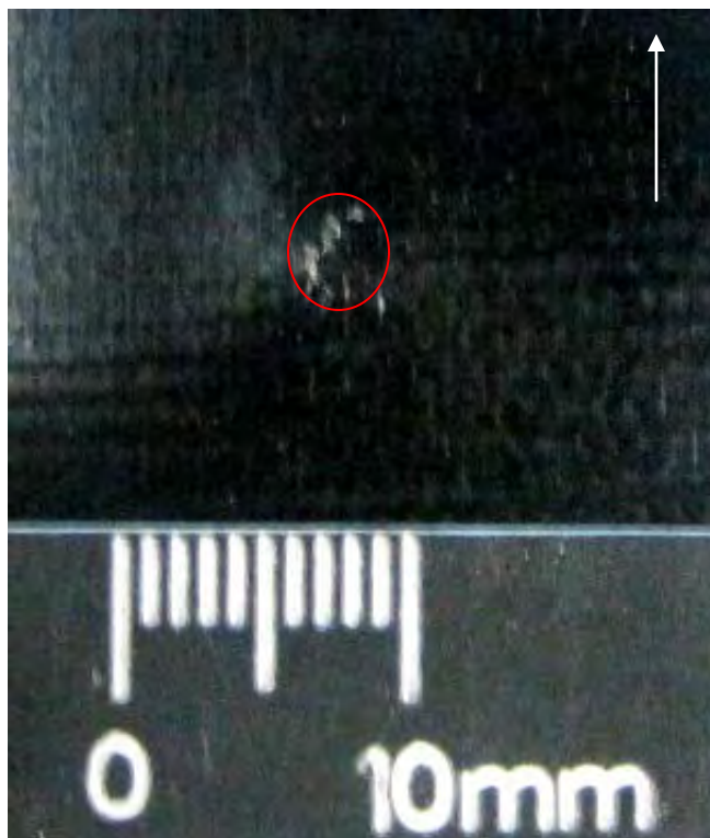
Figure 31 Close-up View of Damage to Back Side of NP 504 Substrate (scale in 1mm increments / white arrow indicates flight path of projectile)
