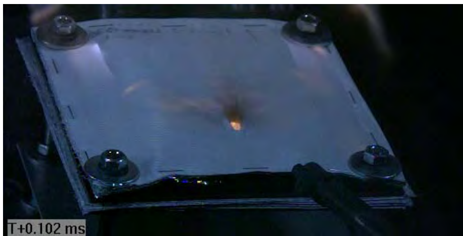
Figure C59 Projectile Impacting Target (via Phantom v711)
