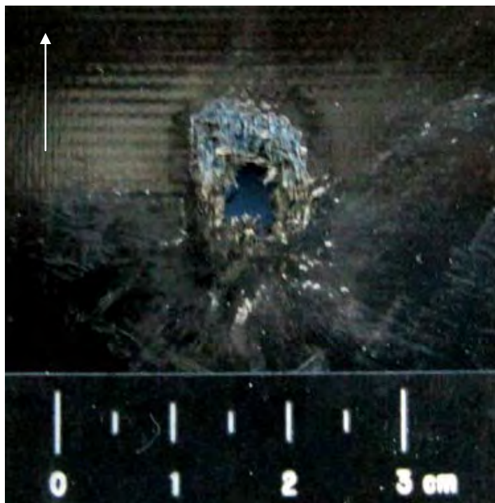
Figure 220 Close-up View of Damage to Front of NP 504 Substrate (scale in 5mm increments / white arrow indicates flight path of projectile)
