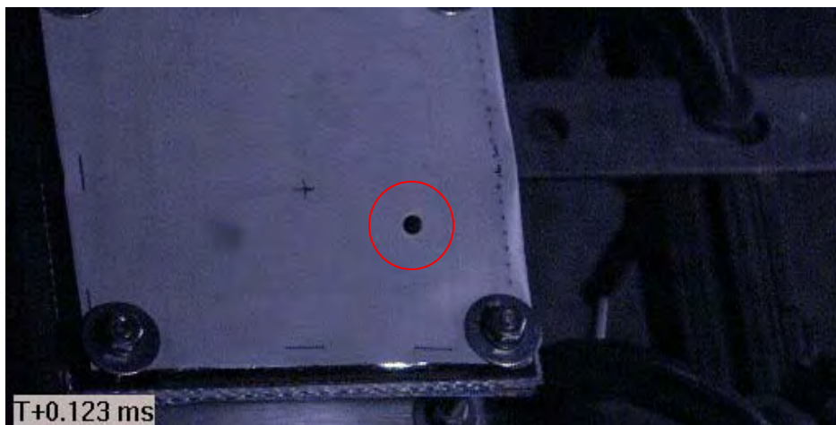
Figure C96 Image of Projectile Captured Prior to Impact (via Phantom v711 / projectile within red circle)
