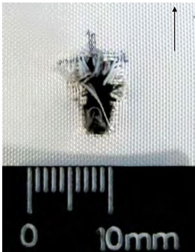
Figure 311 Close-up View of Damage to Front of MLI (scale in 1mm increments / black arrow indicates flight path of projectile)
