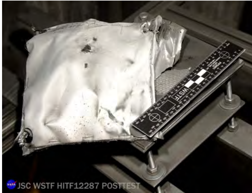
Figure 66 Overall View of Sample in the Target Tank (post-test)
