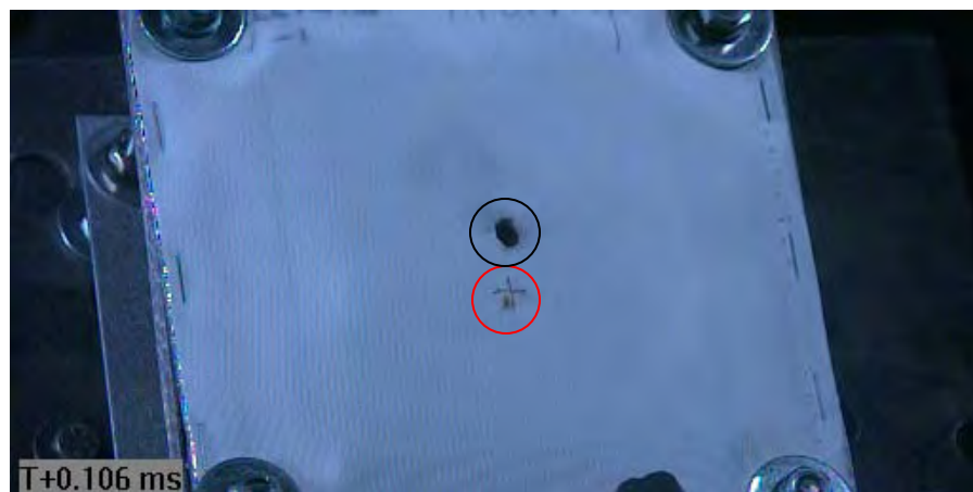
Figure C17 Image of Projectile and Sabot Petal Impacting Target (via Phantom v711 / projectile impact within red circle / sabot petal impact within black circle)
