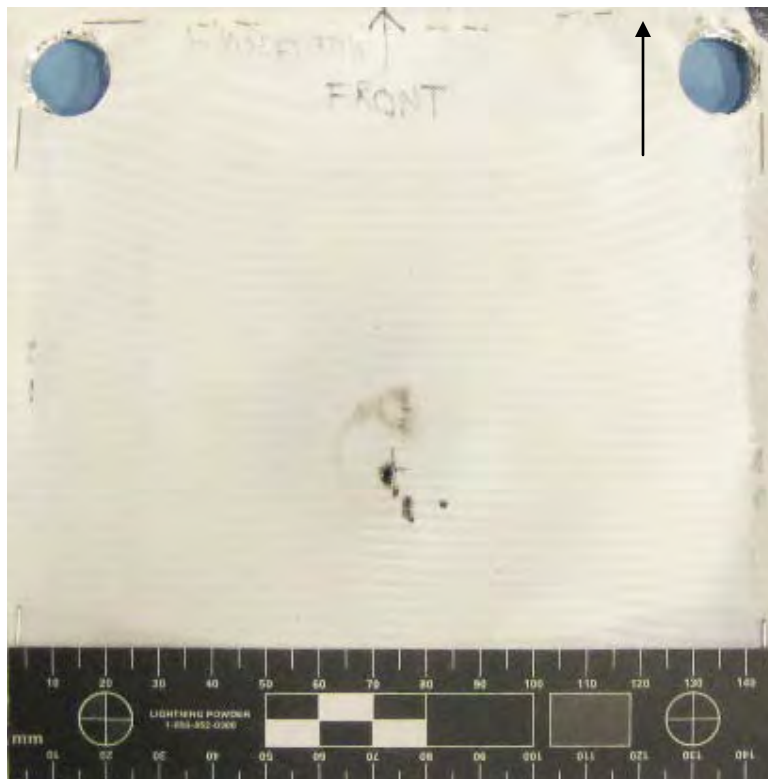
Figure 357 Overall View of Damage to Front of MLI (scale in 5mm increments / black arrow indicates flight path of projectile)
