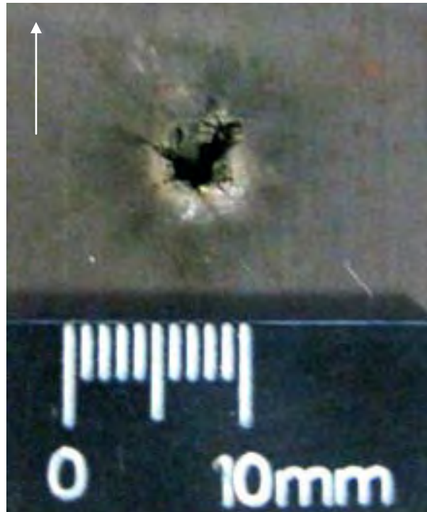
Figure 511 Close-up View of Exit Damage to TORLON 503 (scale in 1mm increments / white arrow indicates flight path of projectile)
