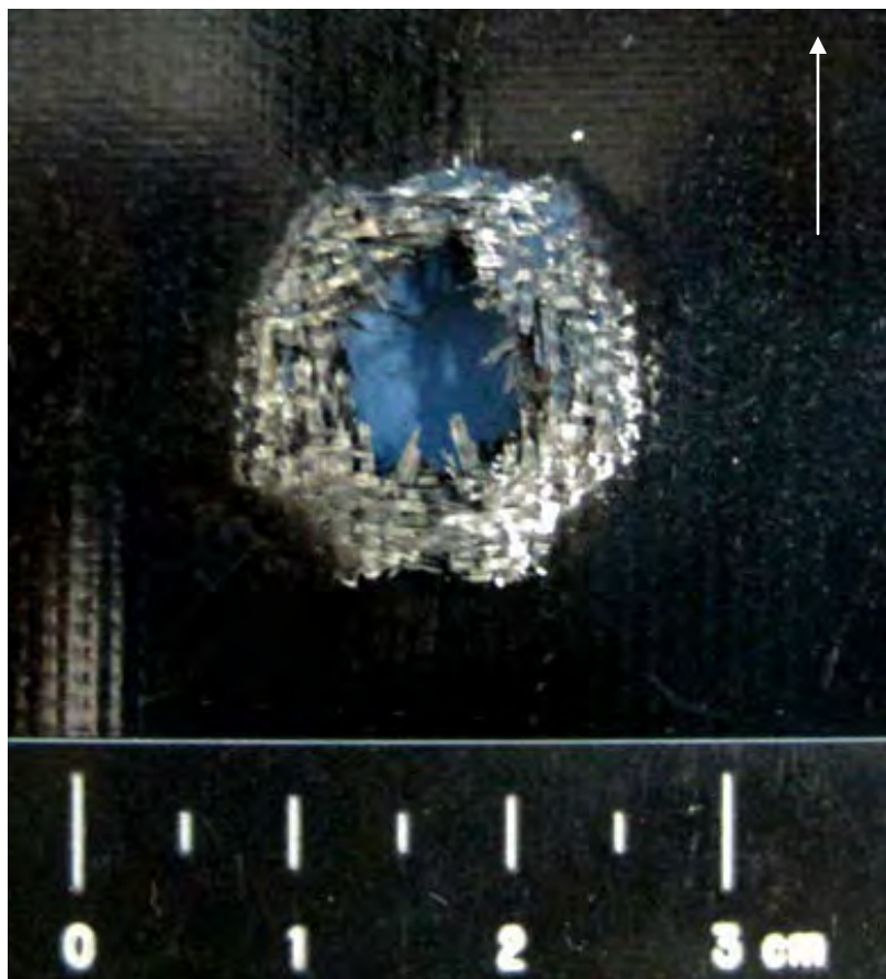
Figure 477 Close-up View of Damage to Back Side of NP 504 Substrate (scale in 5mm increments / white arrow indicates flight path of projectile)
