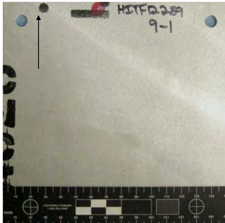
Figure 121 Overall View of Damage to Front of Rear Wall (scale in 5mm increments / black arrow indicates flight path of projectile)
