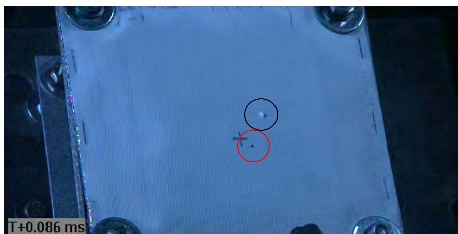
Figure C16 Image of Projectile and Sabot Petal Captured Prior to Impact (via Phantom v711 / projectile within red circle / sabot petal within black circle)
