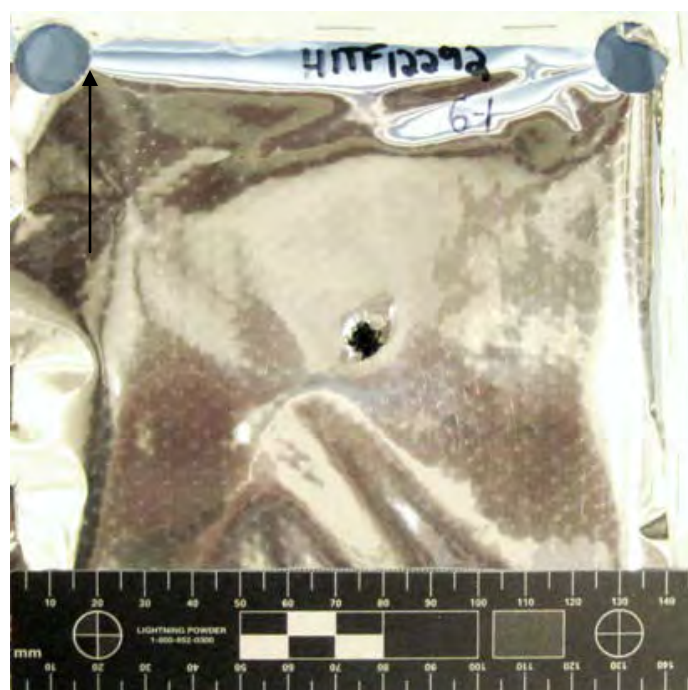
Figure 157 Overall View of Damage to Back Side of MLI (scale in 5mm increments / black arrow indicates flight path of projectile)
