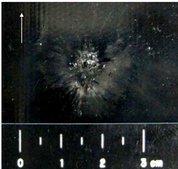
Figure 44 Close-up View of Damage to Front of NP 504 Substrate (scale in 5mm increments / white arrow indicates flight path of projectile)
