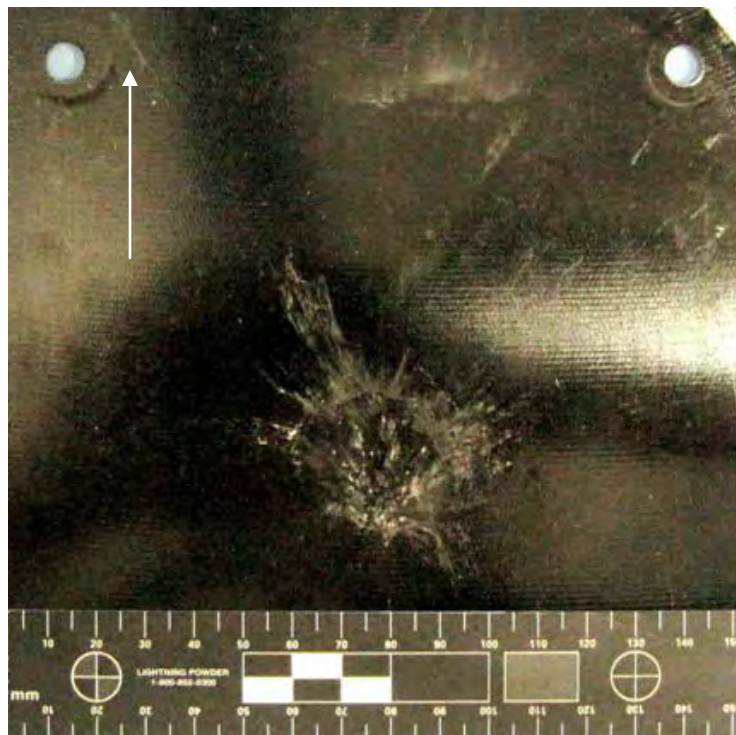
Figure 314 Overall View of Damage to Front of NP 504 Substrate (scale in 5mm increments / white arrow indicates flight path of projectile)
