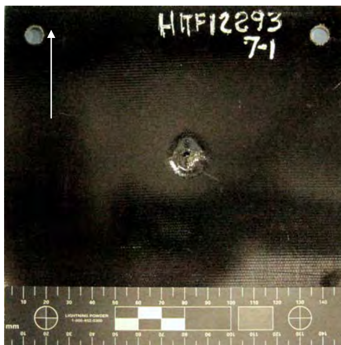
Figure 176 Overall View of Damage to Back Side of NP 504 Substrate (scale in 5mm increments / white arrow indicates flight path of projectile)
