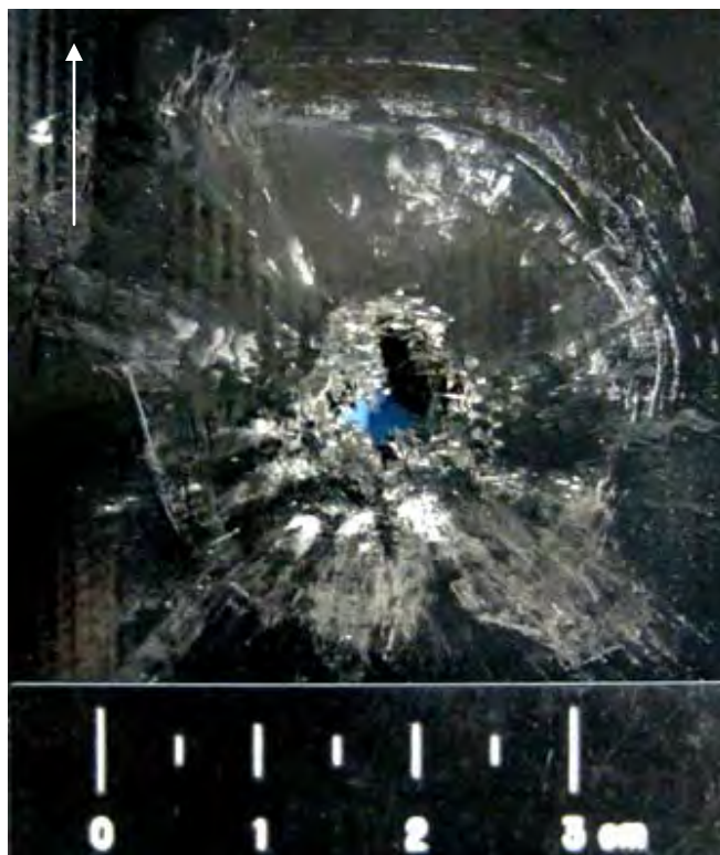
Figure 344 Close-up View of Damage to Front of NP 504 Substrate (scale in 5mm increments / white arrow indicates flight path of projectile)
