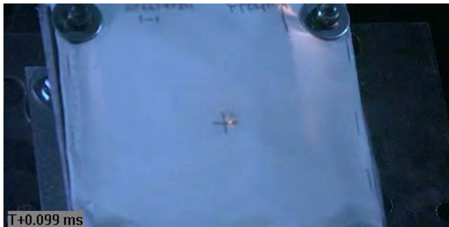
Figure C3 Projectile Impacting Target (via Phantom v711)
