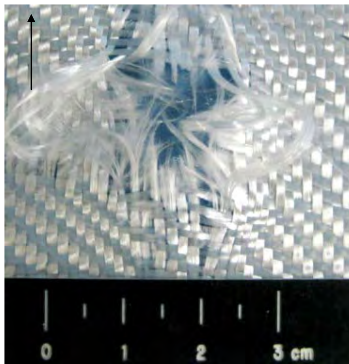
Figure 331 Overall View of Damage to Back Side of Last Fiberglass Layer (scale in 5mm increments / black arrow indicates flight path of projectile)
