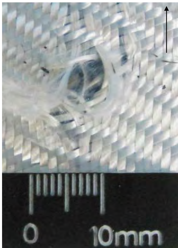
Figure 118 Overall View of Damage to Back Side of Last Fiberglass Layer (scale in 1mm increments / black arrow indicates flight path of projectile)
