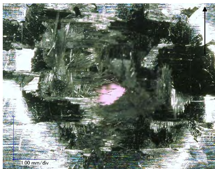
Figure 287 Close-up View of Most Significant Damage to Back Side of NP 504 Substrate (black arrow indicates flight path of projectile / damage within red circle in Figure 286)
