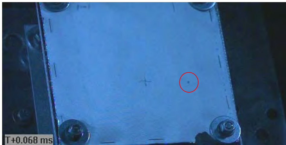
Figure C19 Image of Projectile Captured Prior to Impact (via Phantom v711 / projectile within red circle)
