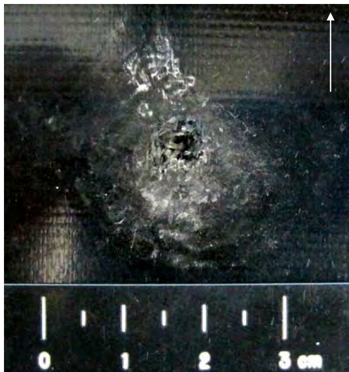
Figure 112 Close-up View of Damage to Front of NP 504 Substrate (scale in 5mm increments / white arrow indicates flight path of projectile)
