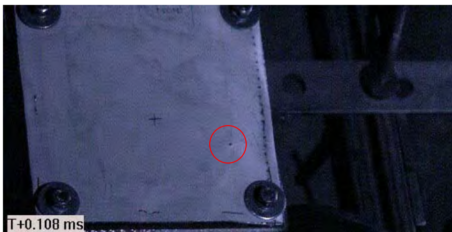
Figure C93 Image of Projectile Captured Prior to Impact (via Phantom v711 / projectile within red circle)
