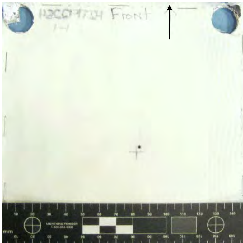
Figure 24 Overall View of Damage to Front of MLI (scale in 5mm increments / black arrow indicates flight path of projectile)
