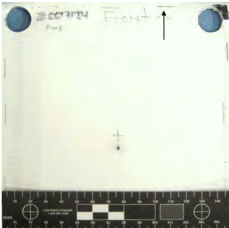
Figure 39 Overall View of Damage to Front of MLI (scale in 5mm increments / black arrow indicates flight path of projectile)
