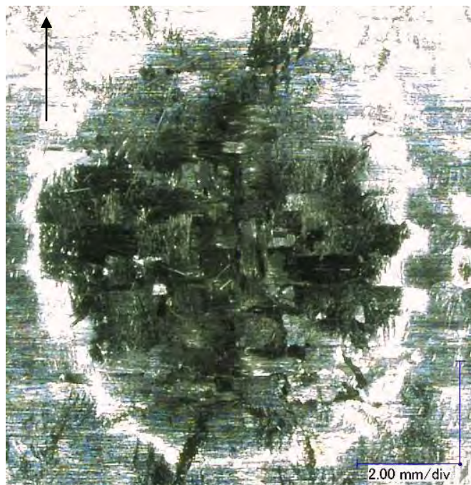
Figure 497 Close-up View of Most Significant Damage to Back Side of NP 504 Substrate (black arrow indicates flight path of projectile / damage within red circle in Figure 496)
