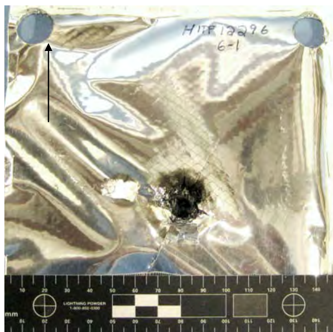
Figure 217 Overall View of Damage to Back Side of MLI (scale in 5mm increments / black arrow indicates flight path of projectile)
