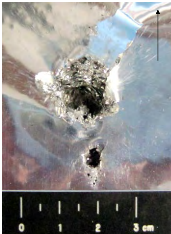
Figure 91 Close-up View of Damage to Back Side of MLI (scale in 5mm increments / black arrow indicates flight path of projectile)
