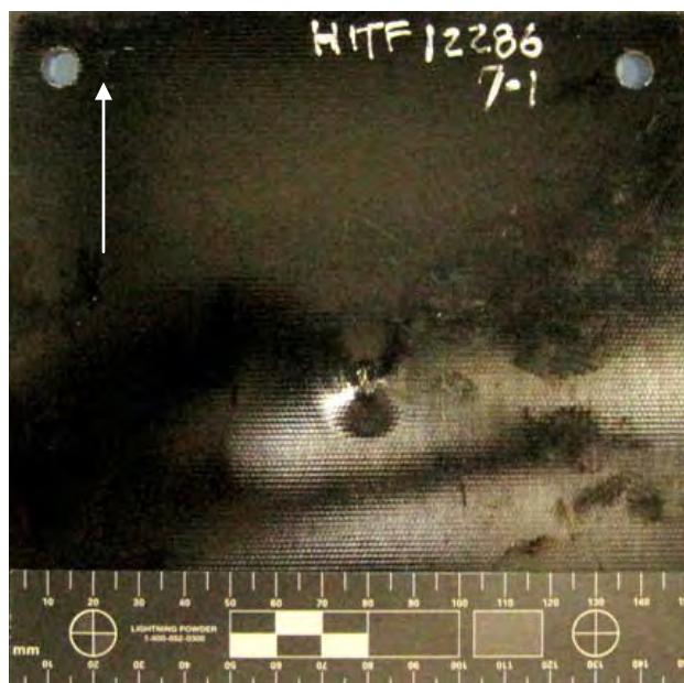
Figure 60 Overall View of Damage to Back Side of NP 504 Substrate (scale in 5mm increments / white arrow indicates flight path of projectile)
