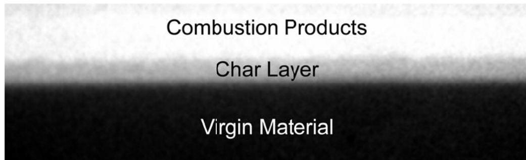
Figure 3-9 X-ray radiograph of charred ablative material
