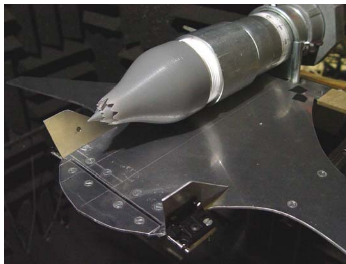
Fig. 3.2.5 Photos of experimental configurations with combination (AC+W18) nozzle. (a) No verticals; (b) nominal verticals; (c) alternate verticals.
