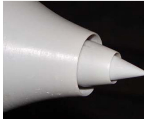
Fig. 3.2.3 Coordinates and picture of BPR10 nozzle
