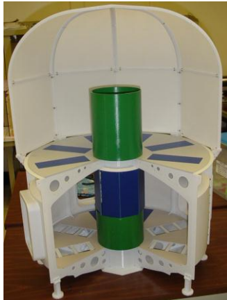
Figure 10 – 1/8 Scale model of the HDU DSH configuration, highlighting use of repositioned structural panels
