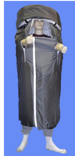
Figure 11 – Full scale model of a wearable water wall based sleeping garment
