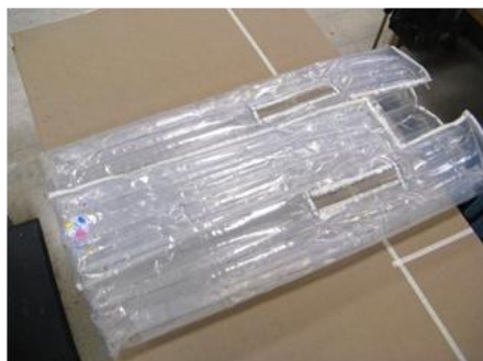
Figure 13 – Water wall bladder insert for the wearable garment
