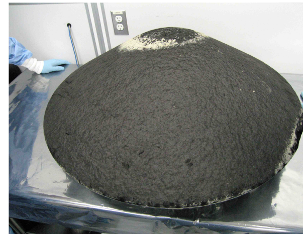
Sample return capsule post-flight with PICA as the forebody TPS. (0.8m diameter)
