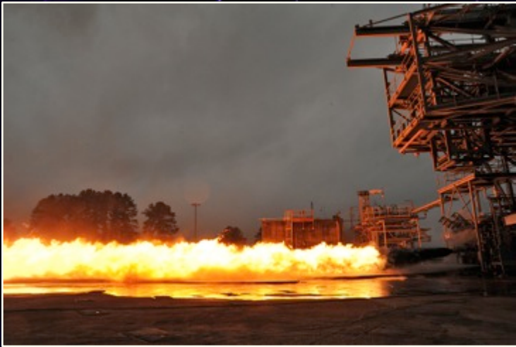
F-1 engine gas generator hot fire test at Marshall Space Flight Center, Jan 2013 – technology development for an optional Advanced Booster concept
