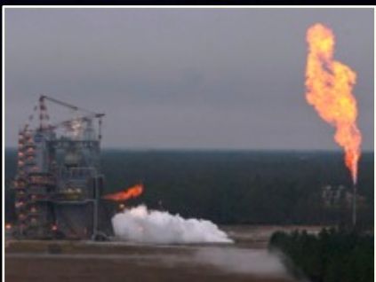
J-2X power pack assembly hot fire test at Stennis Space Center Nov 2012
