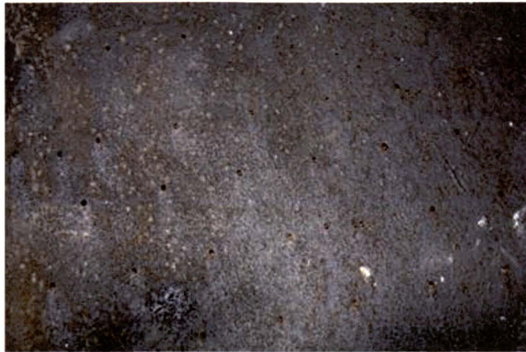
Figure 14. Holes Drilled Into the Surface of the Steel A-2 Test Stand
