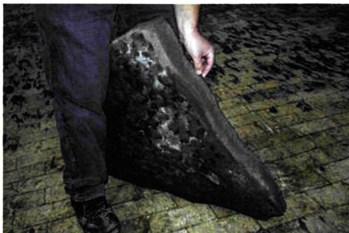
Figure 7. Section of Concrete That was Dislodged During the Launch of STS-126
