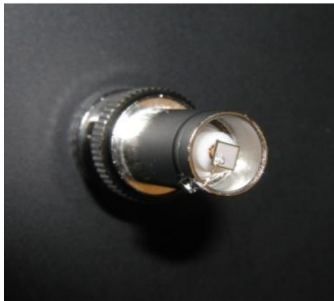
SiC radiation detector for AEVA PCAI studies
