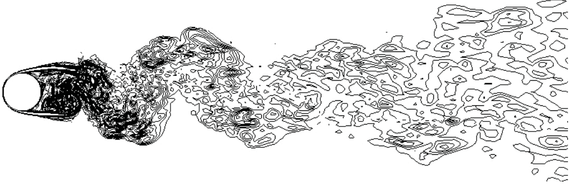
Figure 8: Instantaneous vorticity magnitude \omega D/u_\infty on a x - y plane with 16 contours from \omega D/u_\infty = 0.5 to \omega D/u_\infty = 10.0 in the simulation of v^2 - f DES.
