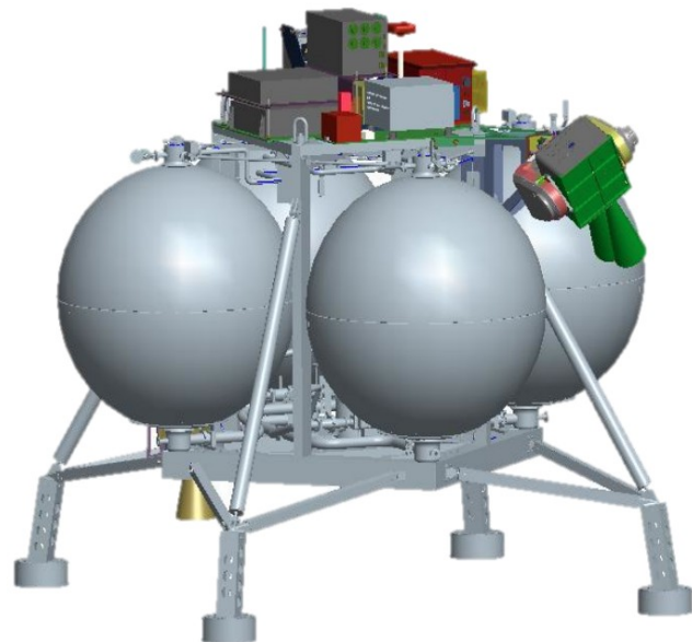
Figure 1. Depiction of the Morpheus flight vehicle with tanks, IMUs, sensors, and engines.
