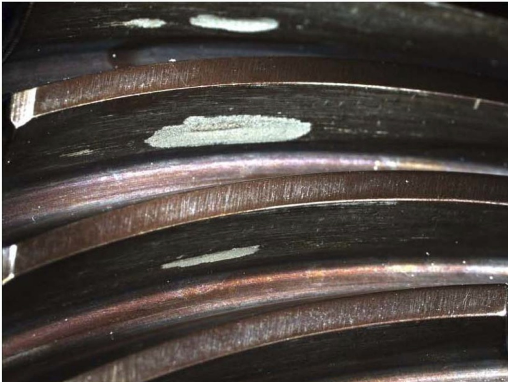
Figure 11.—Output gear damage—progressive pitting.
