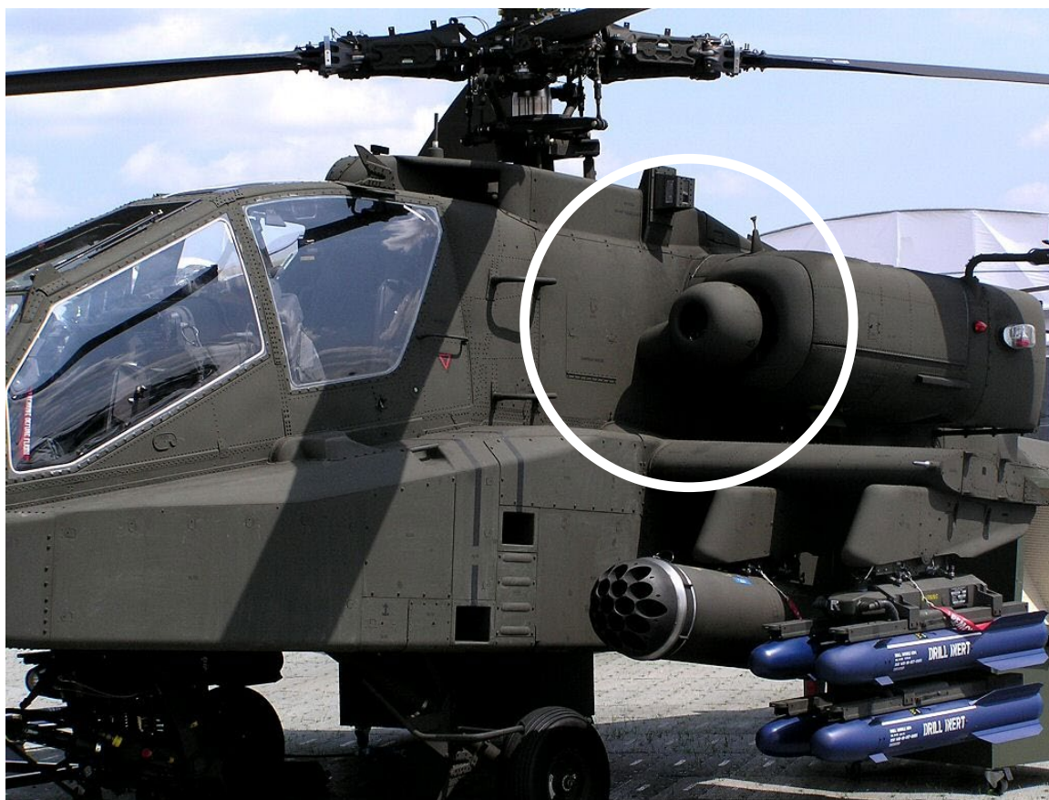
Figure 1.—U.S. Army Helicopter with white circle showing nose gearbox location (Ref. 4).
