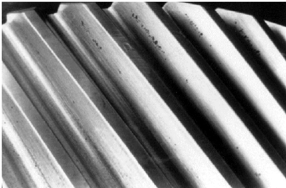
Figure 5.—Example of Initial Pitting. Extracted from ANSI/AGMA 1010-E95, Appearance of Gear Teeth Terminology of Wear and Failure, with the permission of the publisher, the American Gear Manufacturers Association, 1500 King Street, Suite 201, Alexandria, Virginia 22314.
