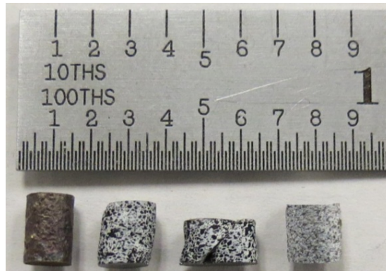
Figure 4.20.—Failure Modes of Ti-6-4 Compression Specimens.
