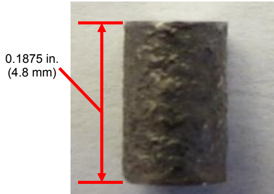
Figure 6.8.—Typical Surface Texturing of As-Cast Ti-6-4 Compression Specimens
