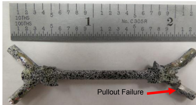
Figure 4.8.—Tensile Failure by Pullout in the Grip.
