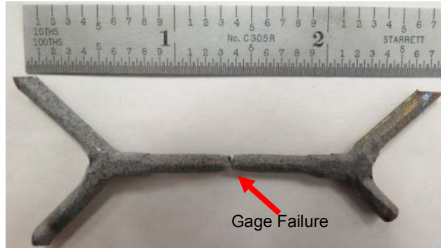
Figure 4.6.—Tensile Failure in the Gage Section.
