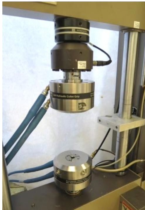
Figure 3.20.—22 kip Servohydraulic Test Frame.
