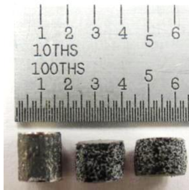
Figure 5.10.—Failure Modes of NiTi Compression Specimens.
