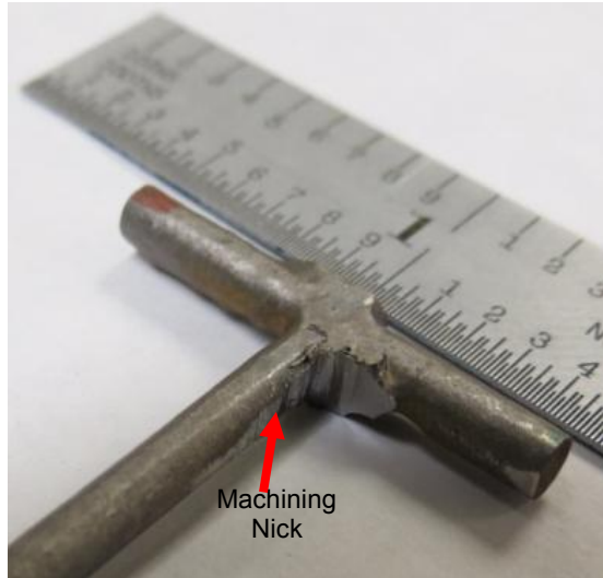
Figure 6.1.—Tensile Specimen with Machining Nick.
