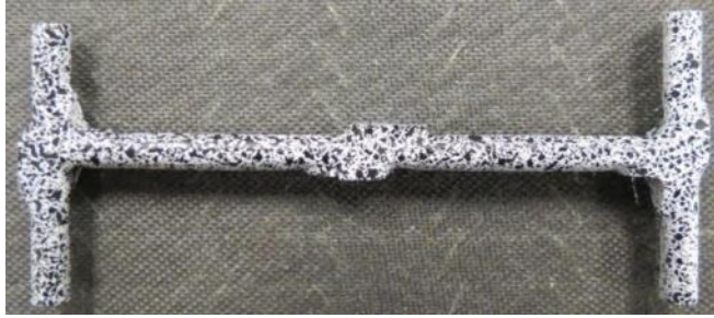
Figure 3.26.—Typical Painted Tension Specimen
