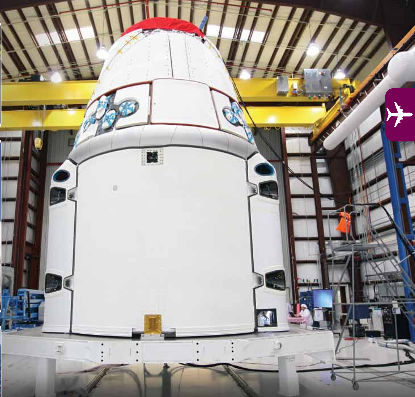
The Space Exploration Technologies', or SpaceX, Dragon spacecraft stands inside a processing hangar at Cape Canaveral Air Force Station in Florida. Engineers install PICA-X tiles on the first Dragon flight's heat shield carrier structure (top inset). On December 8, 2010, the company's Falcon 9 rocket propels Dragon into low Earth orbit for its first test flight (center inset), and, after nearly 3 and a half hours in orbit, the capsule is retrieved after a successful splash down into the Pacific ocean 500 miles off the coast of Mexico (bottom inset).
