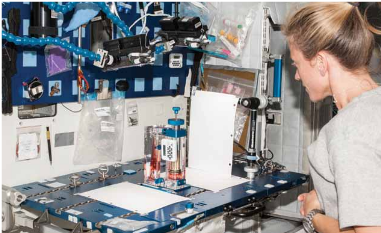
NASA astronaut Karen Nyberg conducts a session with the Capillary Flow Experiment—designed to observe the flow of fluid, in particular capillary phenomena, in microgravity—in the Harmony node of the International Space Station. Accelerometers onboard measure slight gravitational disturbances, which, if left unaccounted for, can skew experiment outcomes.
