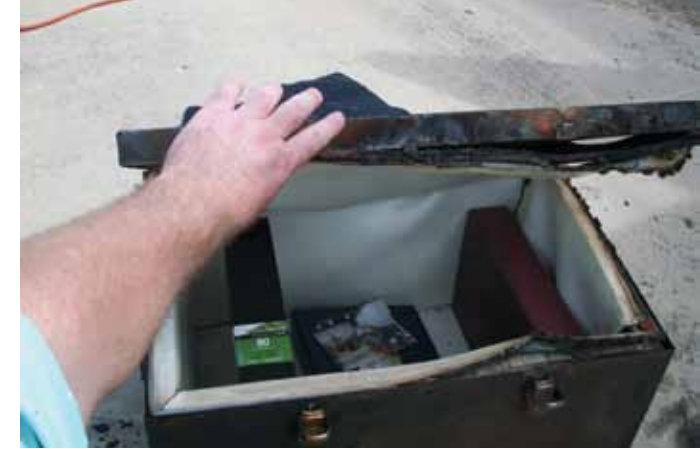
DreamSaver's Home Protection System was constructed with knowledge from a NASA astronaut and engineer who helped to develop the repair techniques for the Space Shuttles' TPS. In the images above, the box is shown before and after a 15-minute burn test at 3,400 °F.
