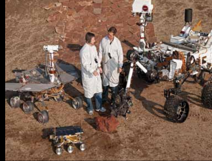
NASA researchers work with full-scale models of various rovers, including Curiosity, in the Jet Propulsion Laboratory's Mars Yard testing area.
