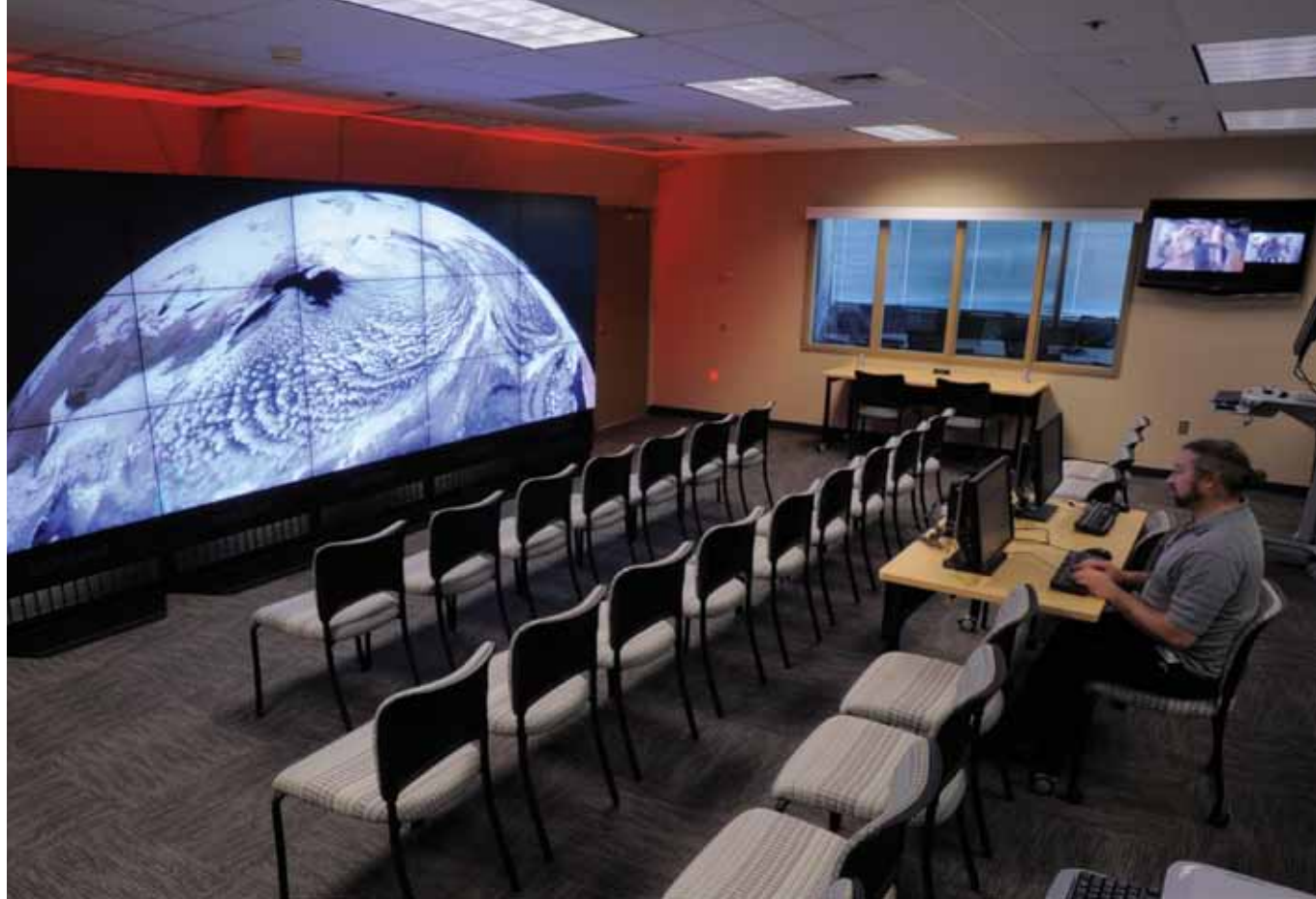
The NASA Center for Climate Simulation Data Exploration Theater features a 17-by-6-foot multi-screen visualization wall for engaging visitors and scientists with high-definition movies of simulation results. Here, the wall displays a 3.5-kilometer-resolution global simulation that captures numerous cloud types at groundbreaking fidelity. Parabon Computation's Frontier Collaborative Online Development Environment, or Frontier CODE, can facilitate both in the development and processing of such a simulation.
