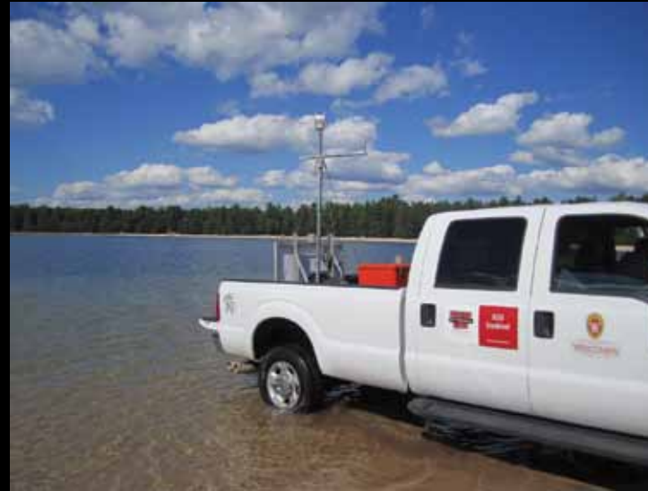
A research team based out of San Diego releases a buoy equipped with sensors into Crystal Lake, Wisconsin. The hardware is running a version of DataTurbine ported to the Android platform, and the team has successfully streamed its real-time data across the country.
