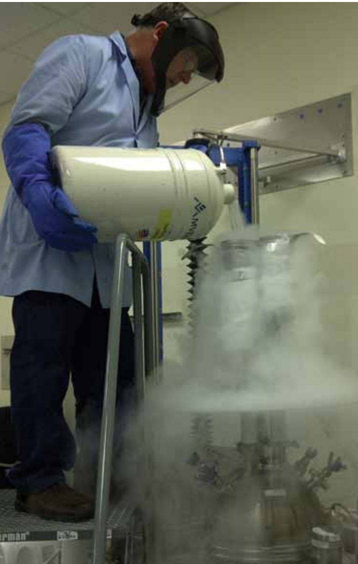
Kennedy Space Center's Wayne Heckle fills a cryostat instrument, developed at the Cryogenics Test Laboratory at Kennedy, with liquid nitrogen. The cryostat instrument tests the thermal performance of insulation materials in a standard, repeatable way.
