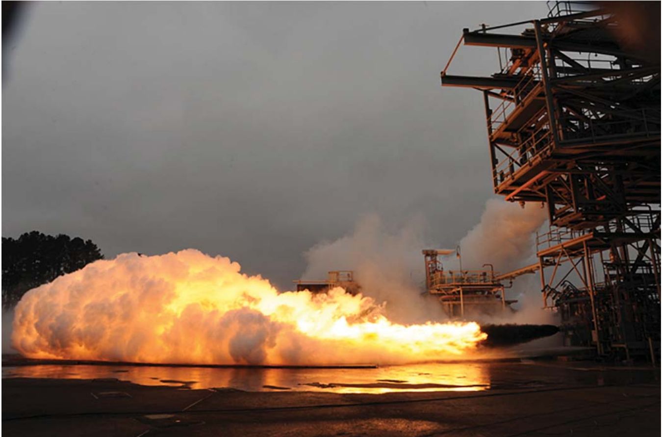
Figure 58. Dynetics ABEDRR GG testing at MSFC.
