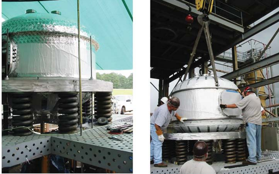
Figure 32. Ullage collapse and capacitance probe test setup (tank mounted at test stand 500).
