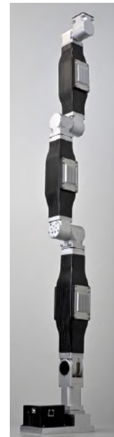
Figure 38. KRAKEN Arm Engineering Model. TUI has delivered an EM unit to NRL for development of advanced arm control methods
