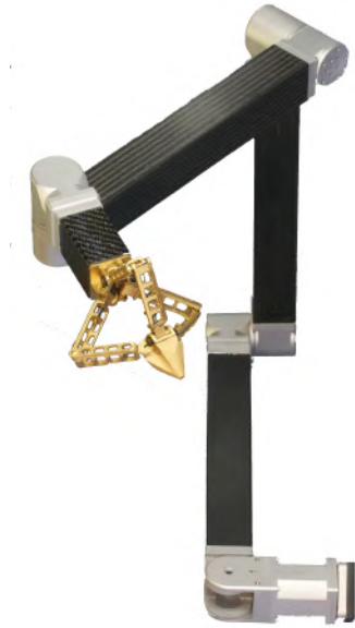
Figure 36. KRAKEN Robotic Arm. The KRAKEN is a 7DOF robotic arm with 1-m reach. Two KRAKEN arms will stow within a 3U CubeSat volume.
