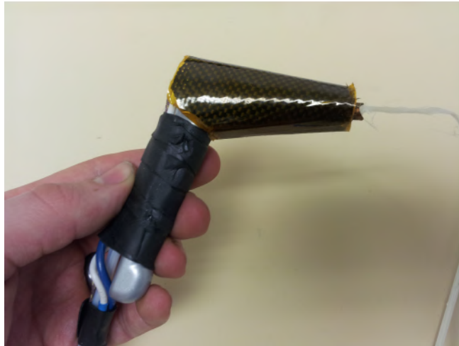
Figure 29. Handheld SpiderFab Pultruder Prototype. We developed and tested manual tools to understand the requirements of the processes that will later be performed robotically.
