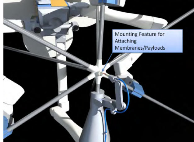
Figure 42. SpiderFab Bot Printing Mounting Feature onto Truss Node. Mounting interface features can be printed onto the joints after completion of the truss structure, which provides another opportunity to compensate for geometry deviations in the placements of the truss members.
